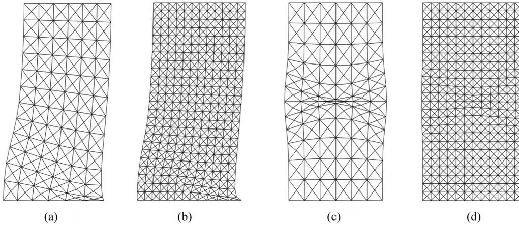
Fig. 4 Deformed shapes (a) imperfection at a corner, 288 elements; (b) imperfection at a corner, 1152 elements; (c) imperfection in the center, 288 elements; (d) imperfection in the center, 1152 elements
