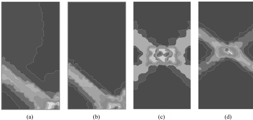
Fig. 3 Contour plots of the equivalent plastic strain (a) imperfection at a corner, 288 elements; (b) imperfection at a corner, 1152 elements; (c) imperfection in the center, 288 elements; (d) imperfection in the center, 1152 elements
