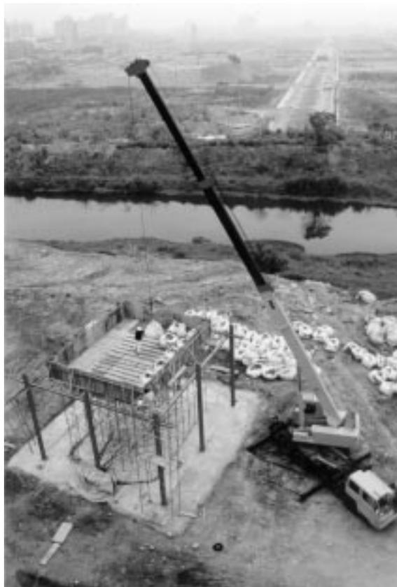
Fig. 5 Outdoor large full-scale loading test of modular falsework under sequential pattern load
