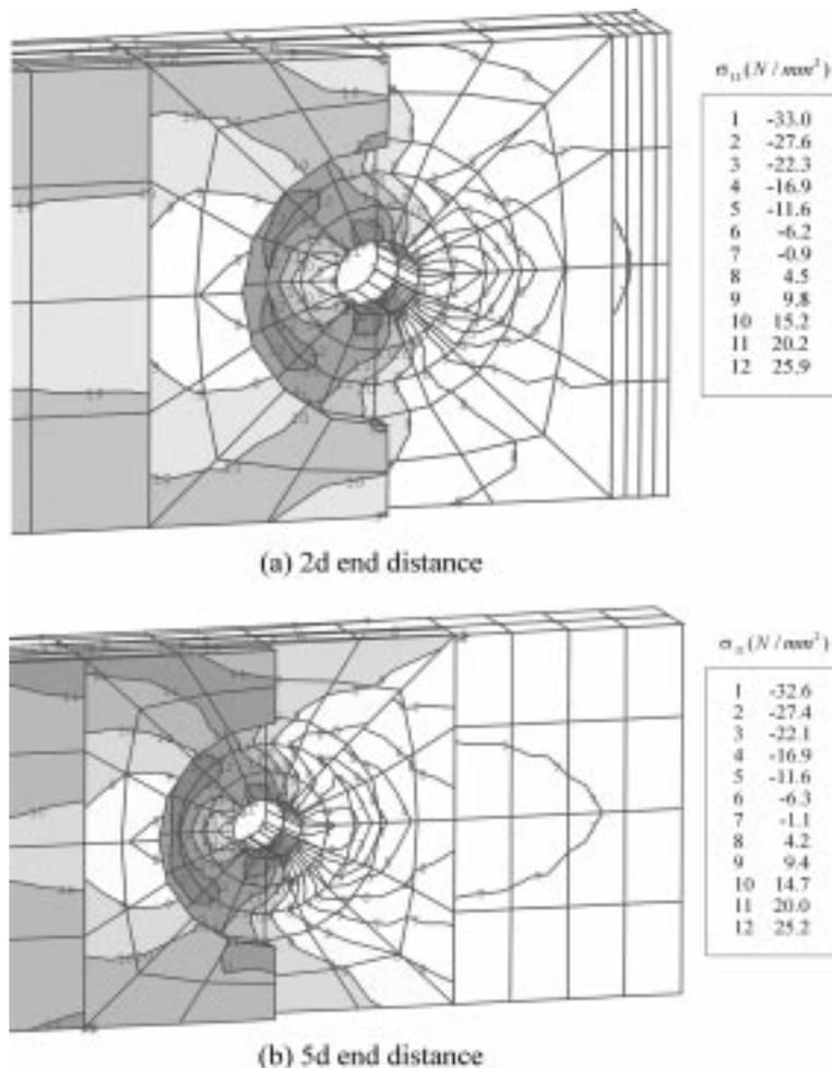
Fig. 10 Typical longitudinal normal stress distributions in the critical areas on the timber member, subjected to changing the end distances
