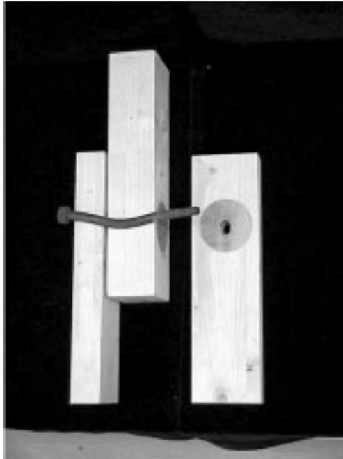
Fig. 1 A timber joint locally reinforced by DVW discs
