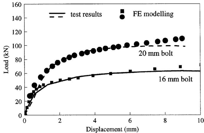
Fig. 4 Load-displacement curves of joints with 16 & 20 mm diameter solid dowels
