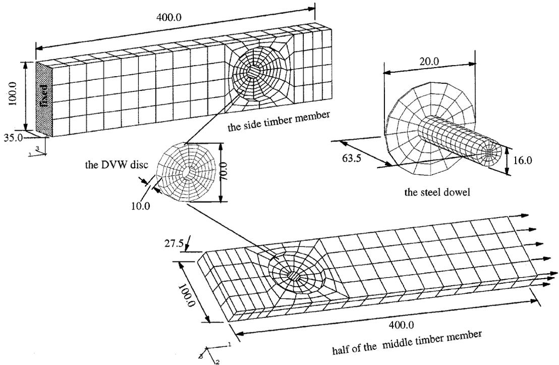
Fig. 3 Mesh generation, loading and boundary conditions for a timber joint locally reinforced by DVW discs
