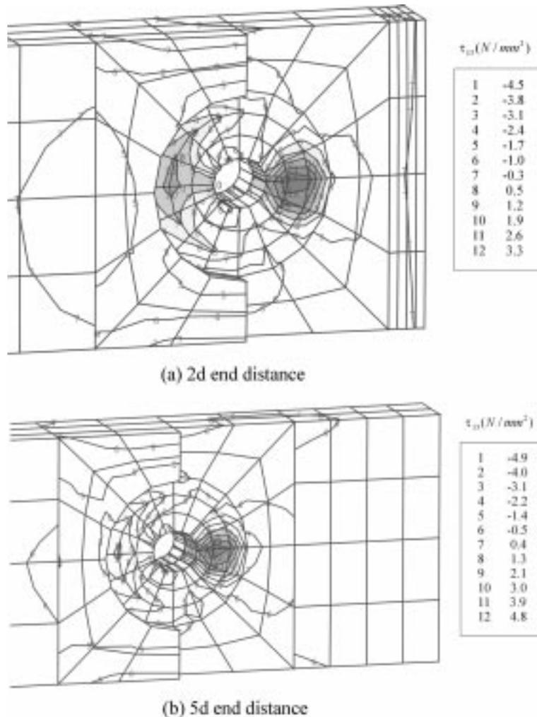
Fig. 11 Typical longitudinal shear stress distributions in the possible failure plane on the timber member, subjected to changing the end distances
