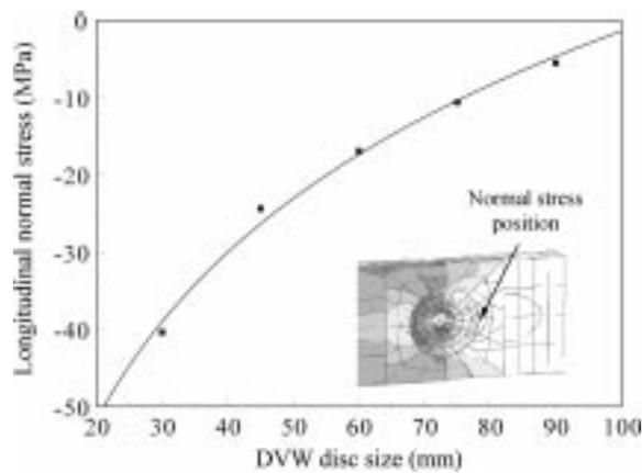
Fig. 7 Variation of the longitudinal normal stresses against DVW disc sizes
