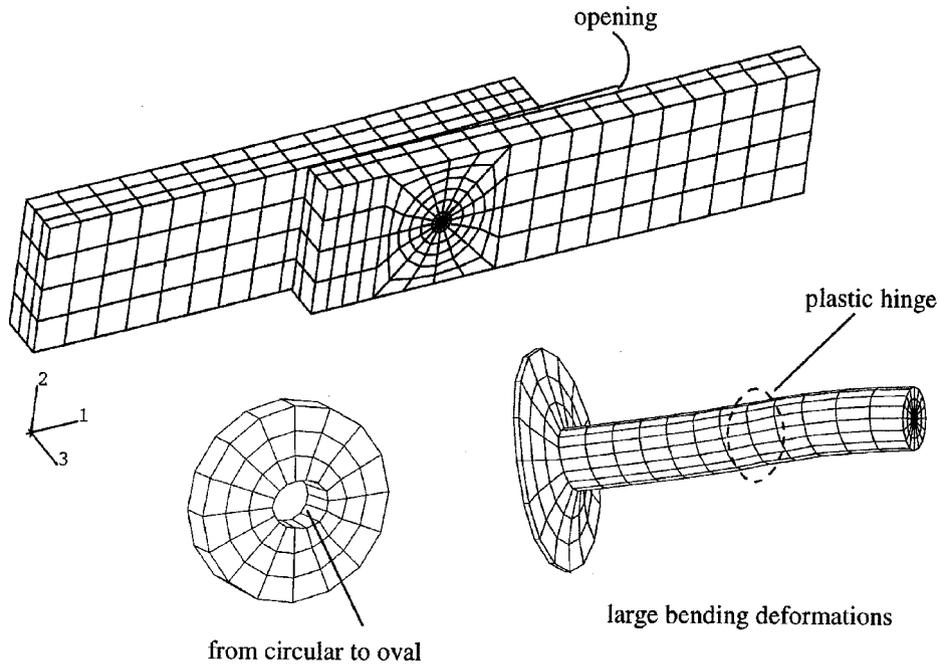
Fig. 5 Displaced meshes of a joint with separate diagrams of the dowel and a DVW disc
