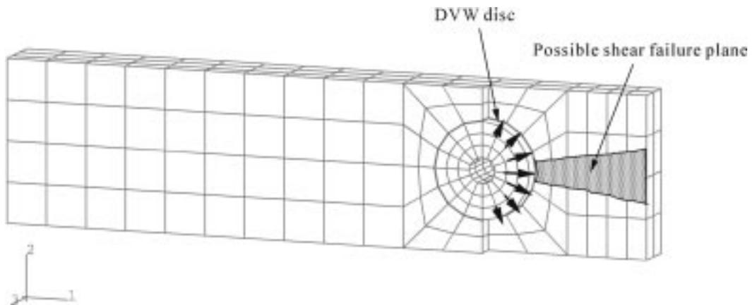
Fig. 2 Possible shear failure plane in the timber member
