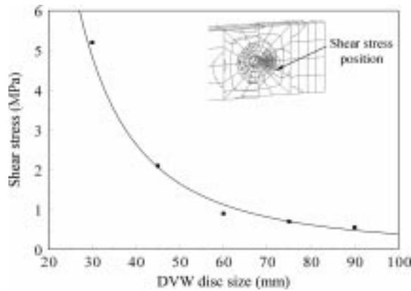
Fig. 9 Variation of the critical longitudinal shear stresses against DVW disc sizes
