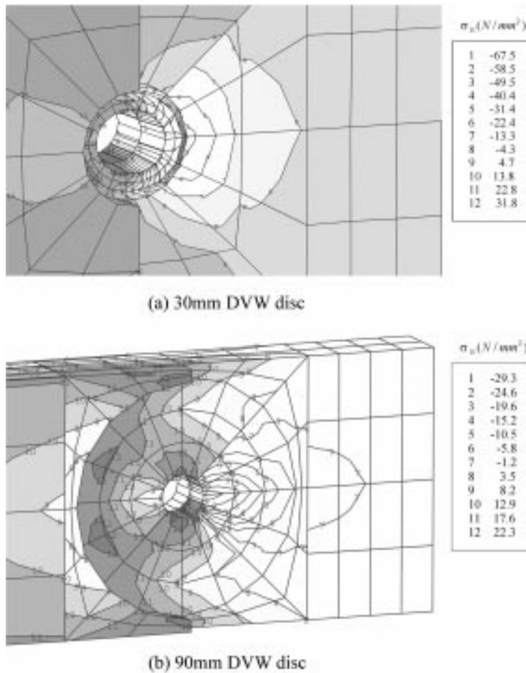
Fig. 6 Typical longitudinal normal stress distributions in the critical areas on the timber member, subjected to changing DVW disc sizes
