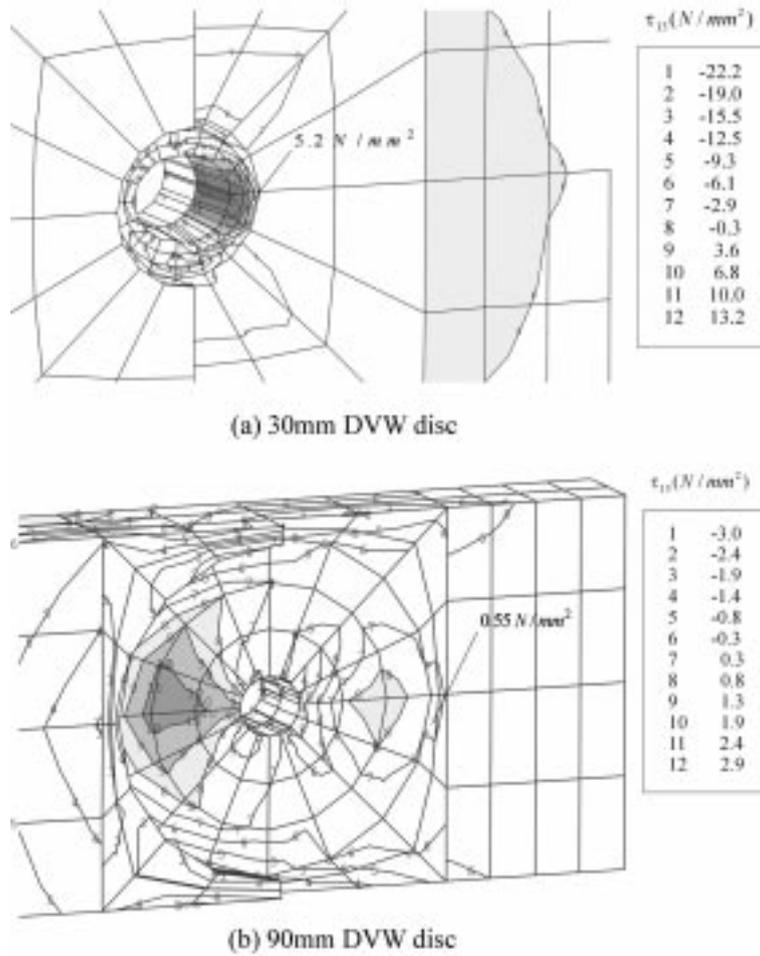
Fig. 8 Typical longitudinal shear stress distributions in the possible failure plane on the timber member, subjected to changing DVW disc sizes
