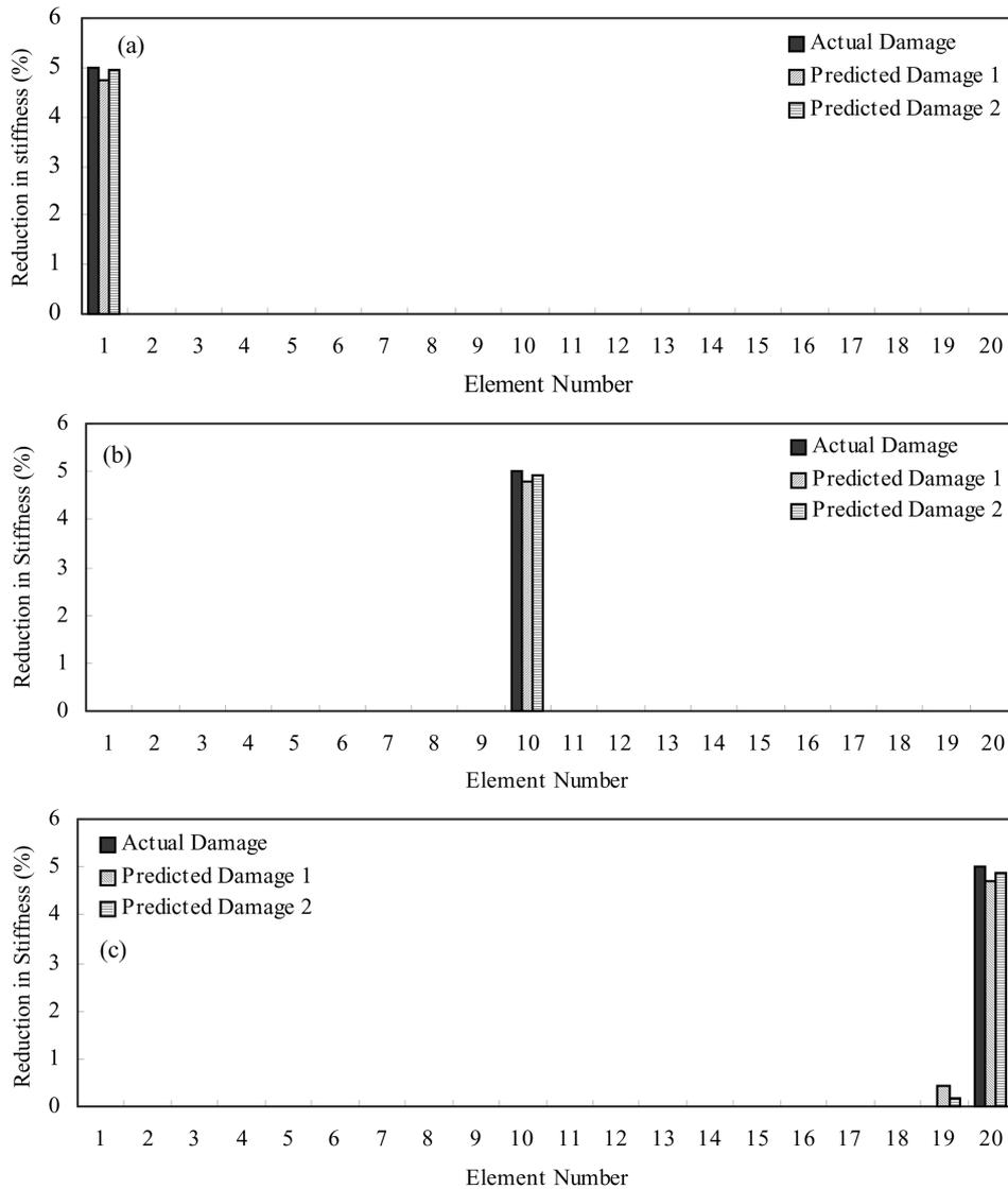
Fig. 4 Detection of light damage of the 20-element periodic spring mass structure without noise injection: (a) Case 1; (b) Case 2; (c) Case 3
