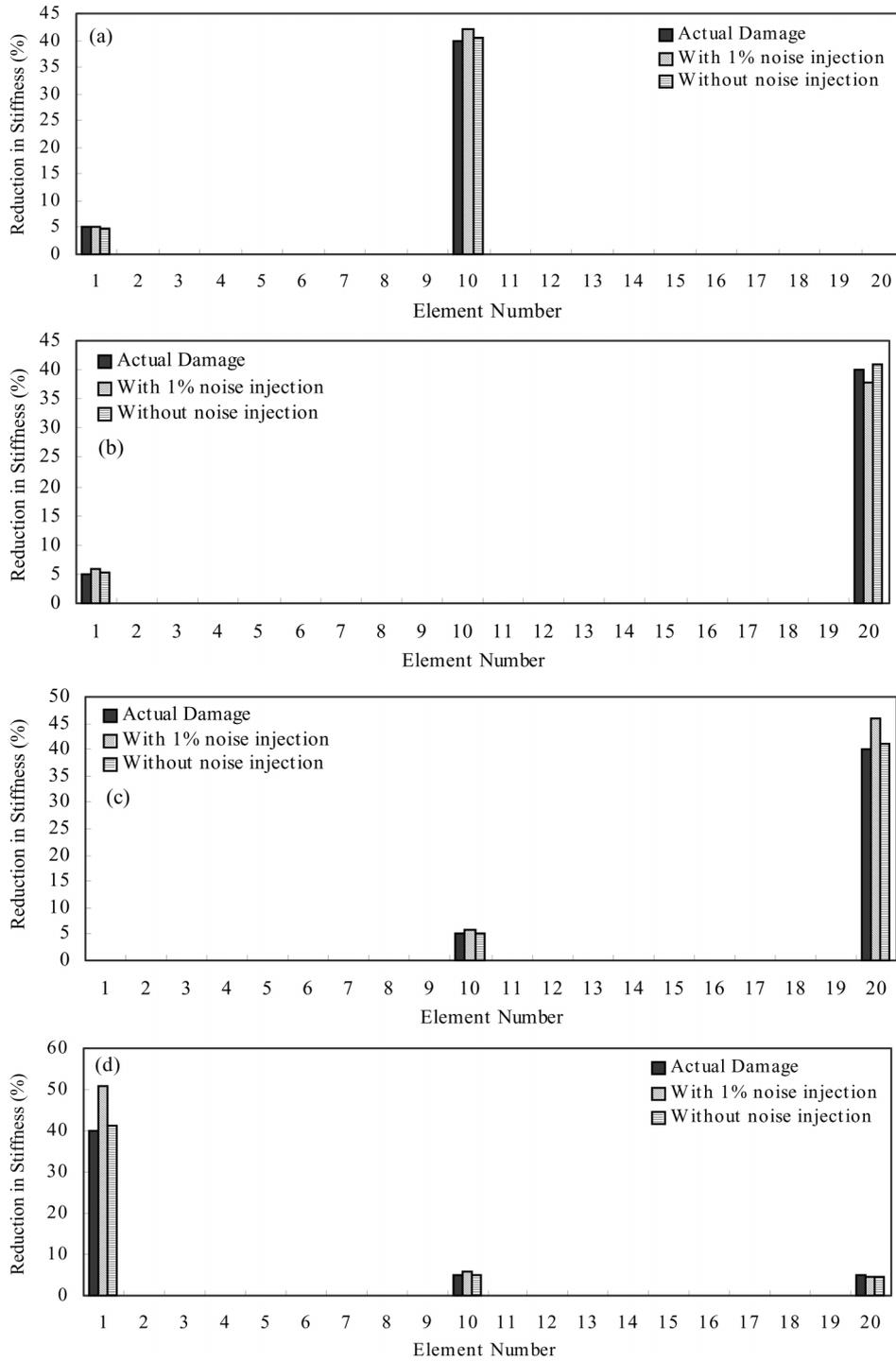
Fig. 7 Detection of multiple damages of the 20-element periodic spring mass structure without and with noise injection by the 2-stage detection method: (a) Case 7; (b) Case 8; (c) Case 9; (d) Case 10
