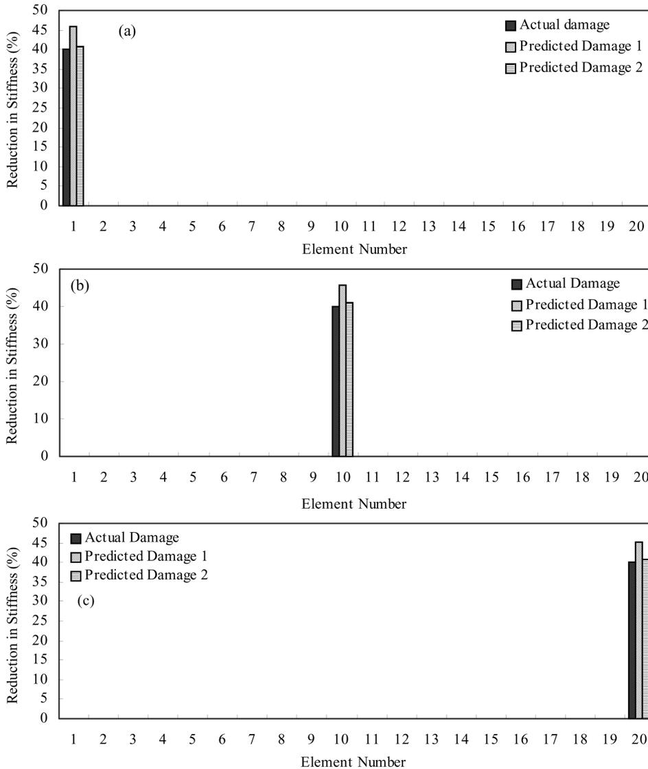
Fig. 5 Detection of severe damage of the 20-element periodic spring mass structure without noise injection: (a) Case 4; (b) Case 5; (c) Case 6
