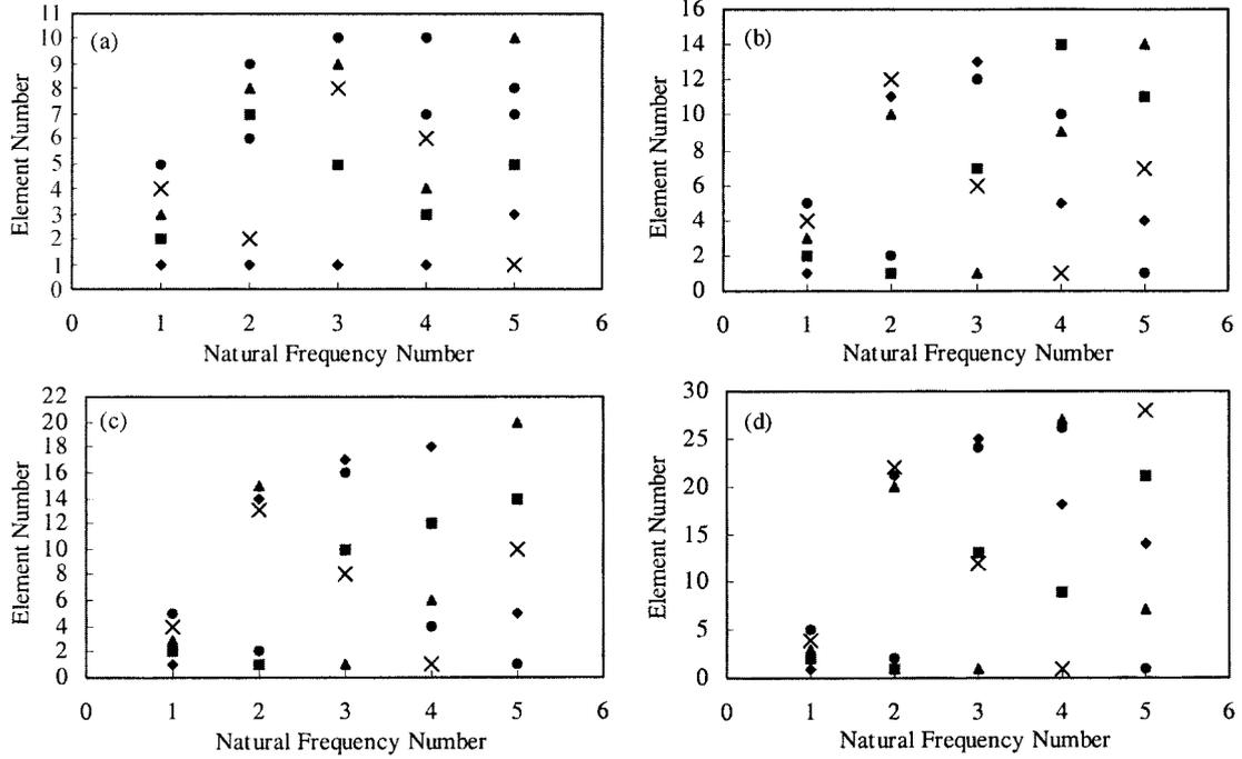
Fig. 3 The 5 locations with the highest damage sensitivities for the first five natural frequencies of the periodic spring-mass systems with different numbers of element: (a)  $N = 10$ ; (b)  $N = 15$ ; (c)  $N = 20$ ; (d)  $N = 30$ .  $\blacklozenge$  the highest;  $\blacksquare$  the second highest;  $\blacktriangle$  the third highest;  $\times$  the fourth highest;  $\bullet$  the fifth highest
