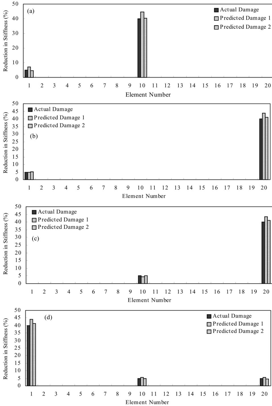
Fig. 6 Detection of multiple damages of the 20-element periodic spring mass structure without noise injection:
