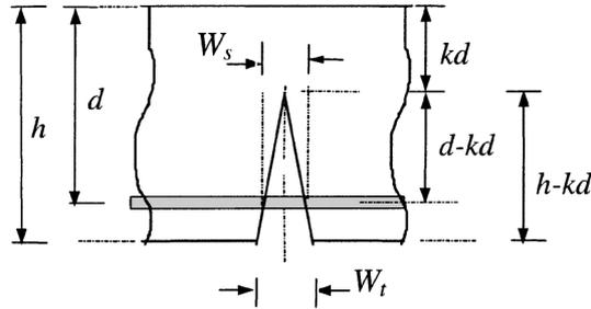
Fig. 4 Relationship between crack widths at reinforcement level and at tension face
