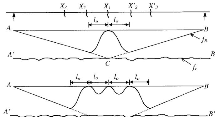
Fig. 10 Propagation of primary cracks in varying moment regions
