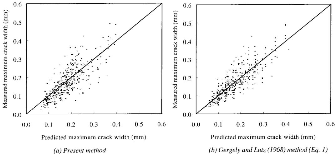
Fig. 14 Comparison of predicted maximum crack width with those measured by Clark (1956) and Chi and Kirstein (1958)
