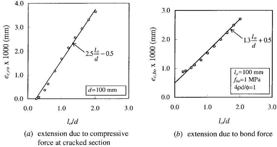
Fig. 2 Approximation for concrete extensions
