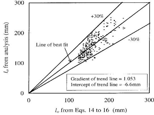
Fig. 6 Comparison of  $l_o$  computed using empirical formulas and 'exact' values
