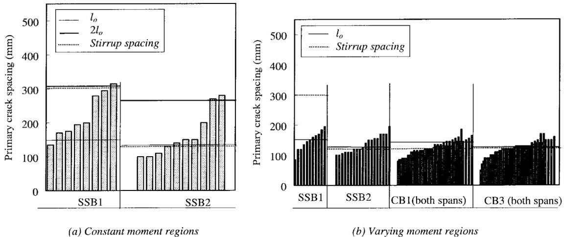
Fig. 11 Comparison of predicted primary crack spacing with those measured by Stewart (1997)
