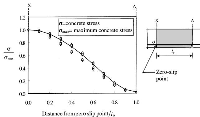
Fig. 7 Variation of concrete stress at the tension face near the first flexural crack
