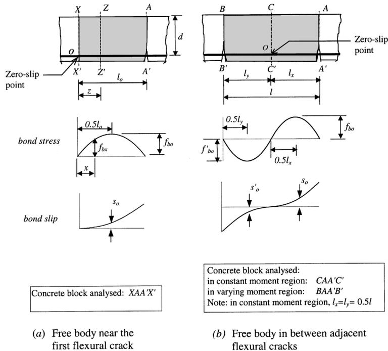
Fig. 1 Details of concrete blocks analysed
