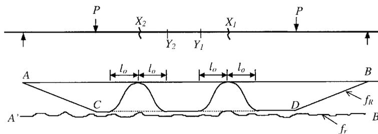
Fig. 9 Propagation of primary cracks in a constant moment region
