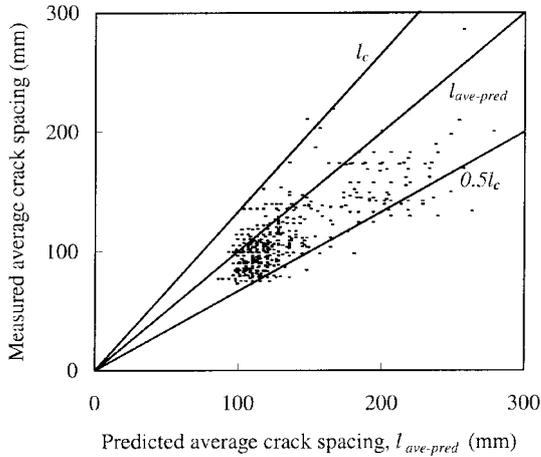
Fig. 12 Comparison of predicted average crack spacing in constant moment regions with those measured by Clark (1956) and Chi and Kirstein (1958)
