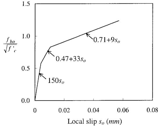
Fig. 3 Bond stress-bond slip relationship used (proposed by Giuriani *et al.* 1991, for deformed bars with stirrups)
