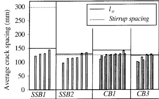
Fig. 13 Comparison of predicted average crack spacing in varying moment regions with those measured by Stewart (1997)
