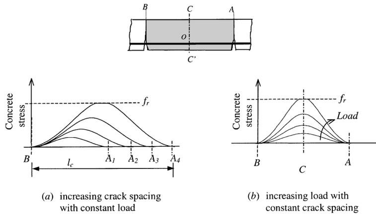
Fig. 8 Variation of concrete tensile stresses at reinforcement level in between adjacent cracks ( $f_r$  = flexural strength of concrete)
