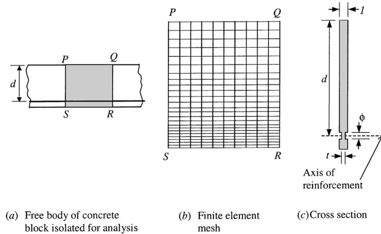
Fig. 5 Finite element mesh and cross section for rectangular beams
