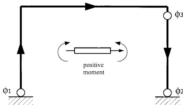
Fig. 4 Introduced hinge locations and sign convention for the first design
