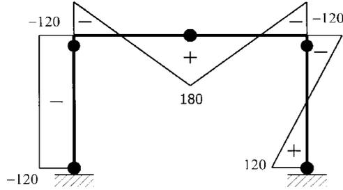
Fig. 6 Bending moment diagram for the optimal solution
