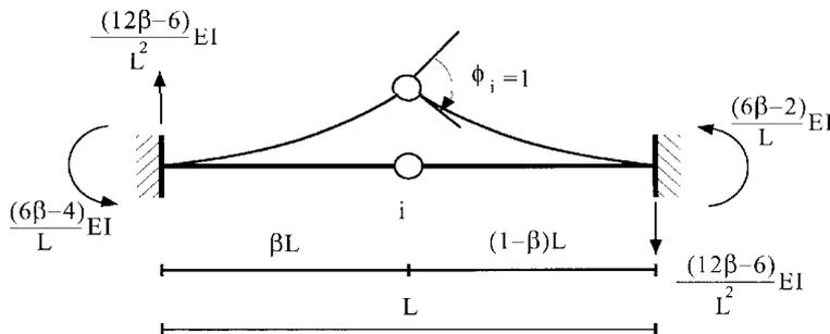
Fig. 1 Fixed end forces of a prismatic member due to the unit introduced hinge rotation
