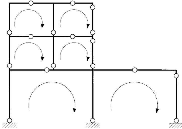
Fig. 2 Automatic generation of introduced hinge locations on a statically indeterminate frame
