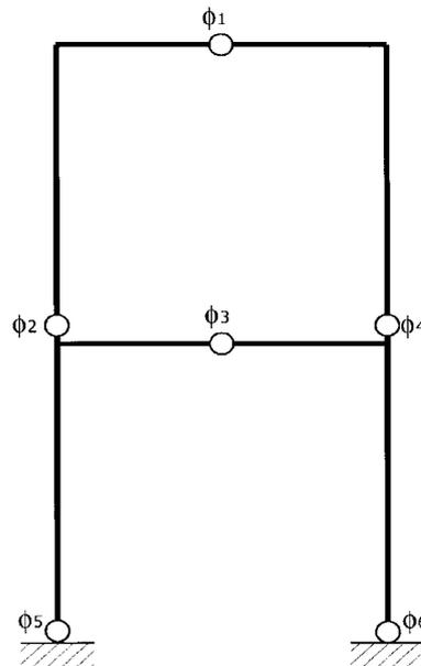
Fig. 10 Statically determinate released frame with introduced hinges
