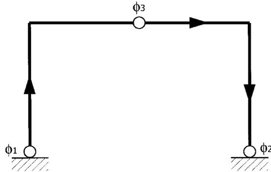
Fig. 5 Introduced hinge locations for the second design
