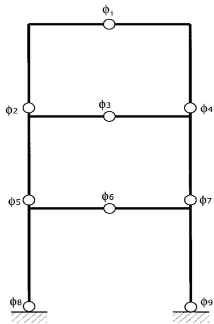
Fig. 12 Statically determinate released frame with introduced hinges
