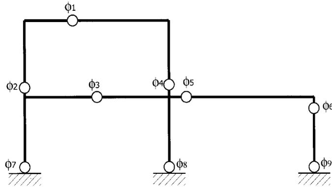
Fig. 8 Introduced hinge locations over the two-bay, two-storey frame
