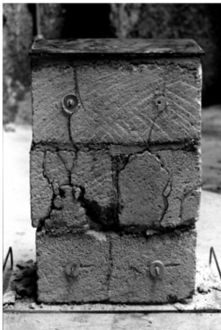
Fig. 4 Cracking picture and failure mode of specimen
