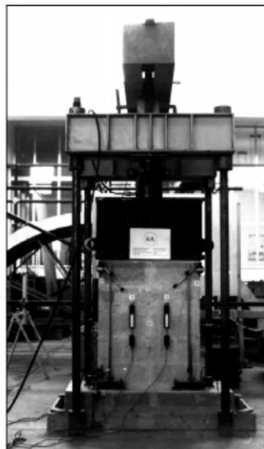
Fig. 2 Masonry specimen and loading arrangement      Fig. 3 Specimen of greater size and loading arrangement
