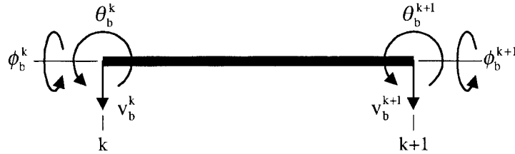
Fig. 4 Degrees of freedom of beam element
