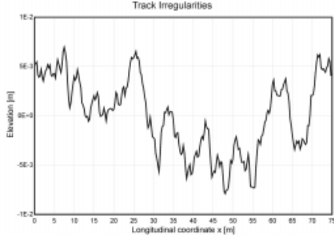
Fig. 6 Track irregularities as longitudinal coordinate x
