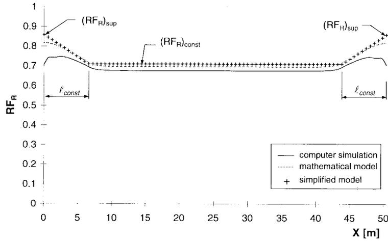
Fig. 4 Simplified shear flow range reduction factors  $RF_R$
