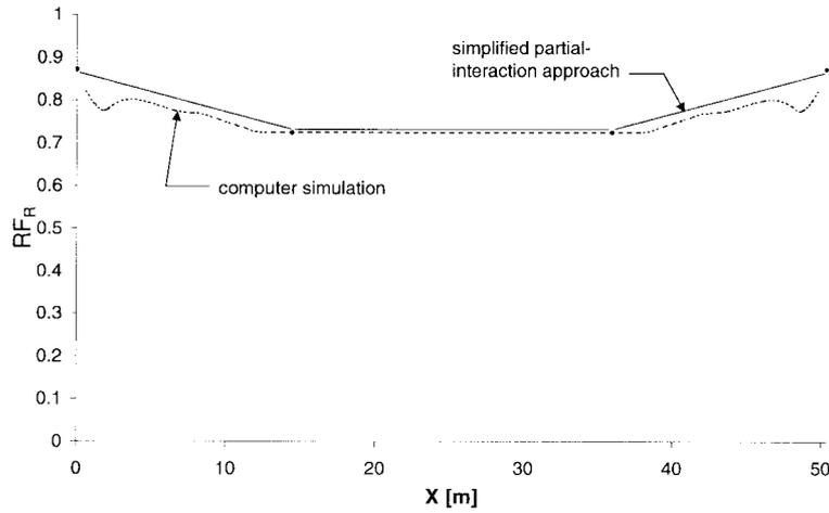
Fig. 6 Partial-interaction distribution of shear flow forces
