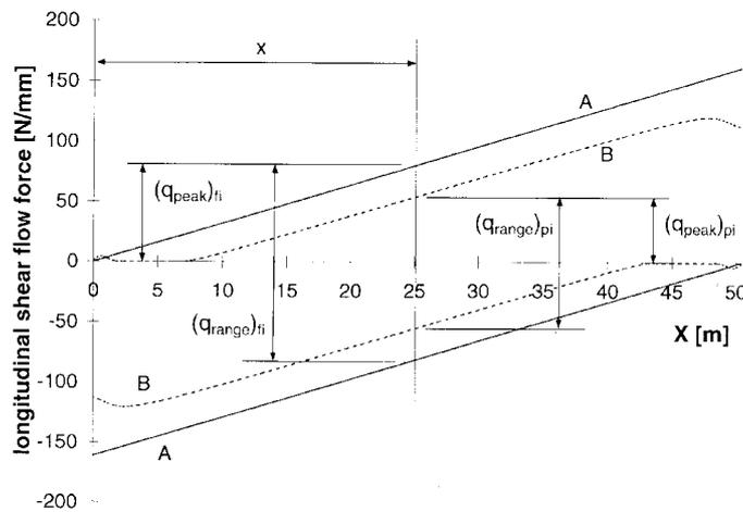
Fig. 3 Shear flow force envelopes for a moving concentrated load
