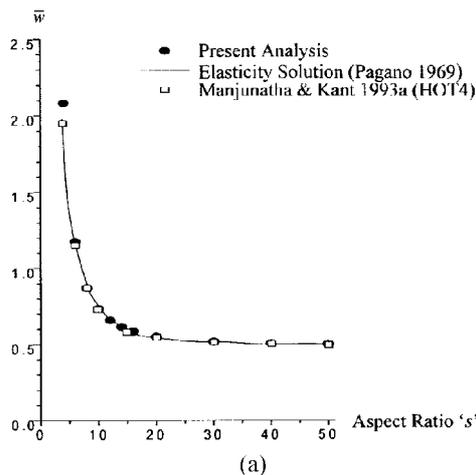
Fig. 2 (a) Variation of normalized transverse displacement ( $\bar{w}$ ) with aspect ratio  $s$  ( $s = a/t$ ) at  $(a/2, 0)$  for a simply supported homogeneous orthotropic beam under sinusoidal loading.
