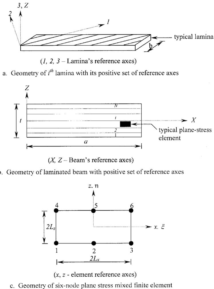
Fig. 1 (a-c) Geometry of laminated beam and mixed finite element
