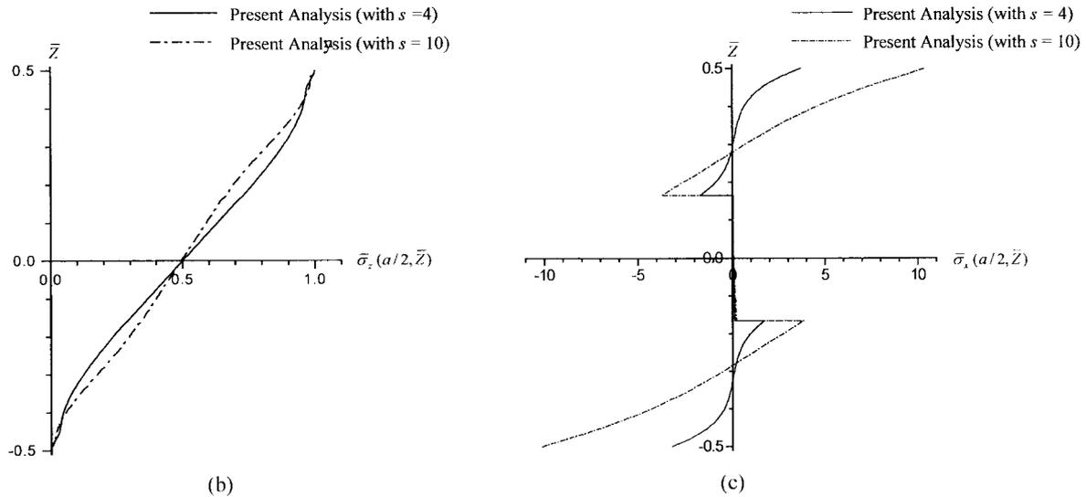
Fig. 5 (b, c) Variation of normalized (b) transverse normal stress ( $\bar{\sigma}_z$ ); and (c) in-plane normal stress ( $\bar{\sigma}_x$ ); through the thickness of cross-ply ( $0^\circ/90^\circ/0^\circ$ ) laminated beams subjected to sinusoidal loading and supported on fixed supports at the ends
