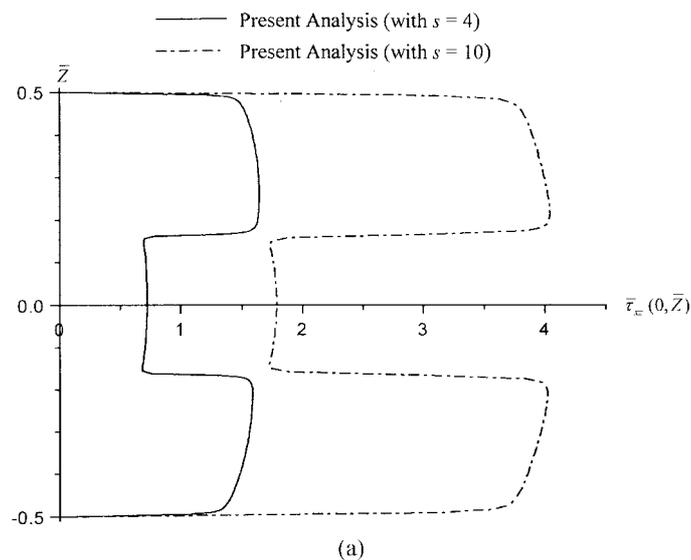
Fig. 5 (a) Variation of normalized (a) transverse shear stress ( $\bar{\tau}_{xz}$ ) through the thickness of cross-ply (0°/90°/0°) laminated beams subjected to sinusoidal loading and supported on fixed supports at the ends
