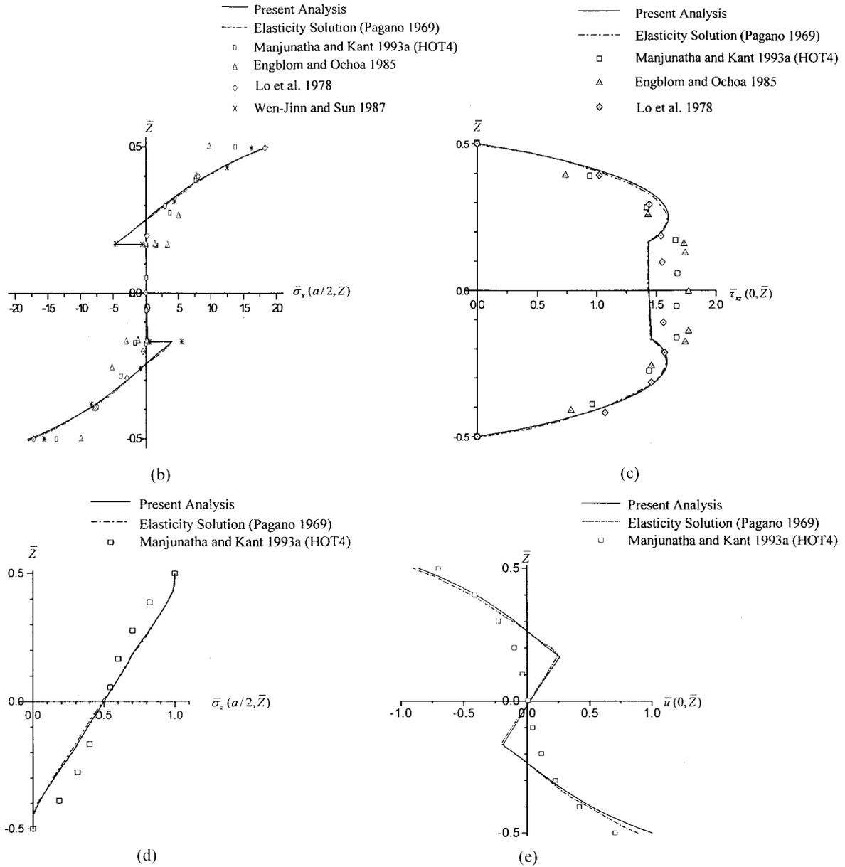
Fig. 4 Variation of normalized (b) in-plane normal stress ( $\bar{\sigma}_x$ ); (c) transverse shear stress ( $\bar{\tau}_{xz}$ ); (d) transverse normal stress ( $\bar{\sigma}_z$ ); and (e) in-plane displacement ( $\bar{u}$ ); through the thickness of a simply supported cross-ply ( $0^\circ/90^\circ/0^\circ$ ) laminated beam ( $s = 4$ ) under sinusoidal loading
