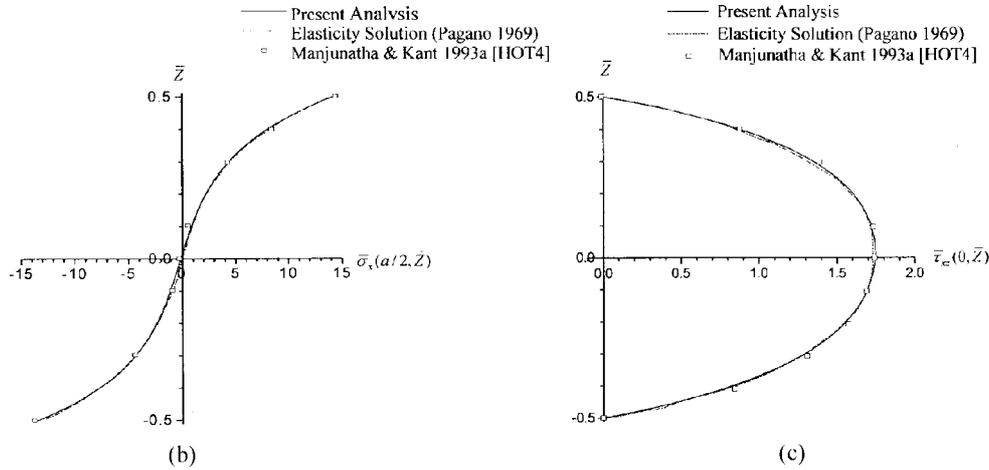
Fig. 2 (b, c). Through-thickness variation of normalized (b) in-plane normal stress ( $\bar{\sigma}_x$ ) and (c) transverse shear stress ( $\bar{\tau}_{xz}$ ) for a simply supported homogeneous orthotropic beam with  $s=4$  under sinusoidal loading
