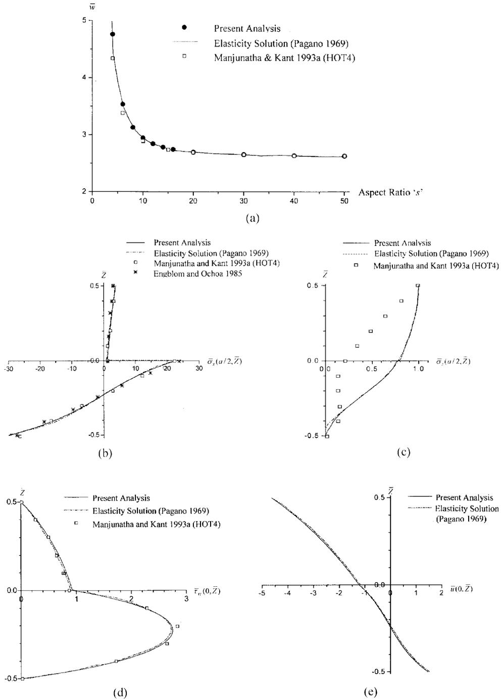
Fig. 3 Variation of normalized (a) transverse displacement ( $\bar{w}$ ) with aspect ratio  $s$  ( $s=a/t$ ) at  $(a/2,0)$ ; (b) in-plane normal stress ( $\bar{\sigma}_x$ ); (c) transverse normal stress ( $\bar{\sigma}_z$ ); (d) transverse shear stress ( $\bar{\tau}_{xz}$ ); and (e) in-plane displacement ( $\bar{u}$ ); through the thickness of a simply supported cross-ply ( $0^\circ/90^\circ$ ) laminated beam with  $s = 4$ , under sinusoidal loading
