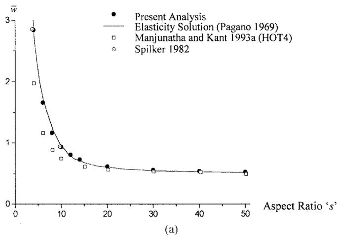
Fig. 4 (a) Variation of normalized transverse displacement ( $\bar{w}$ ) with aspect ratio  $s$  ( $s = a/t$ ) at  $(a/2, 0)$  for a simply supported cross-ply ( $0^\circ/90^\circ/0^\circ$ ) laminated beam under sinusoidal loading
