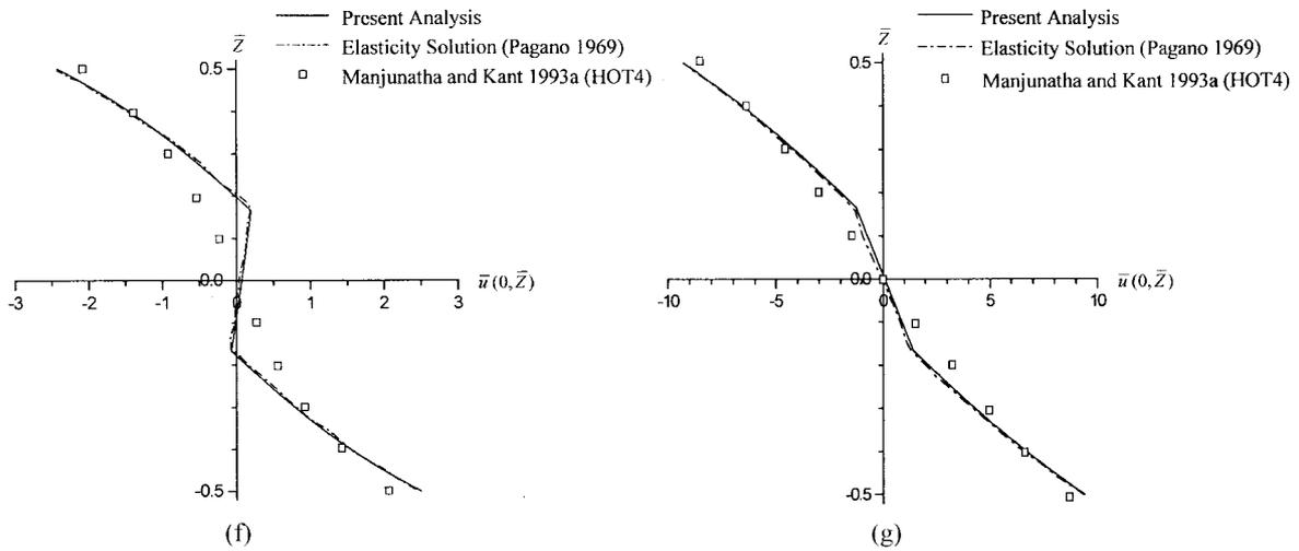
Fig. 4 (f, g) Variation of normalized (f) in-plane displacement ( $\bar{u}$ ) with  $s = 6$ ; and (g) in-plane displacement ( $\bar{u}$ ) with  $s = 10$ ; through the thickness of a simply supported cross-ply (0°/90°/0°) laminated beam under sinusoidal loading
