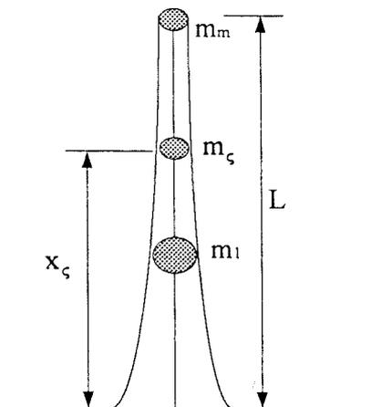
Fig. 3 A Cantilever bar with variable parameters and lumped masses
