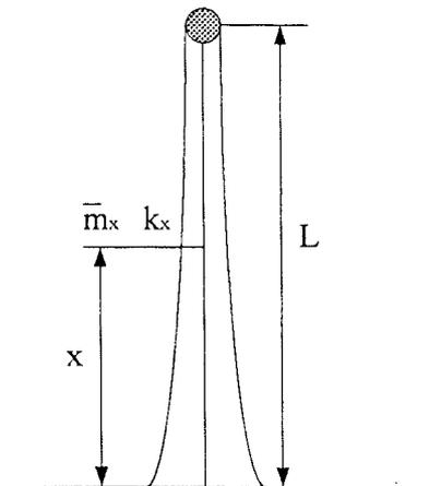
Fig. 1 A Cantilever bar with varying cross-section
