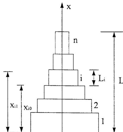
Fig. 2 A multi-step cantilever bar
