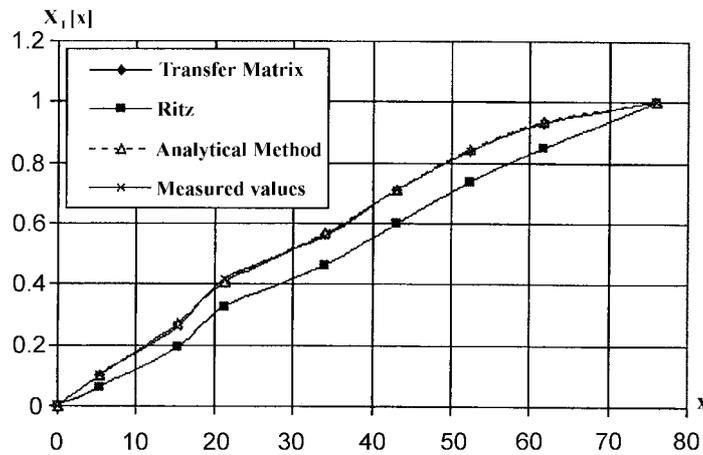
Fig. 6 The fundamental mode shape
