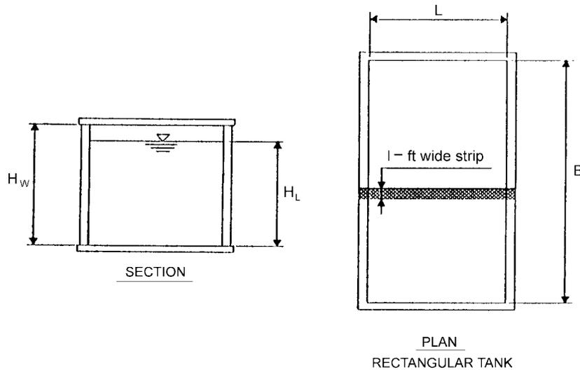
Fig. 3 Dimensions of rectangular tank
