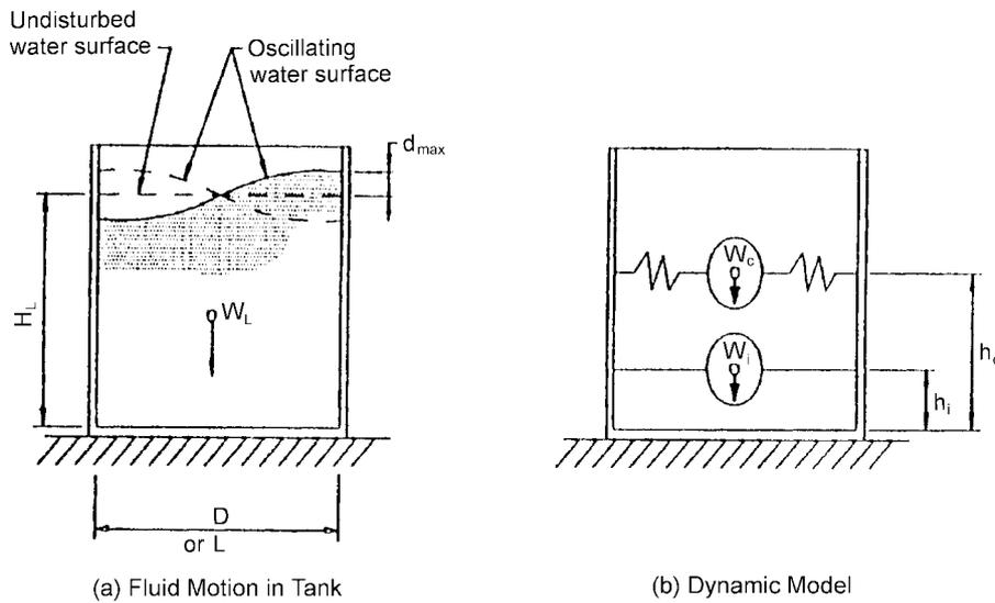
Fig. 1 Dynamic model of liquid-containing tank rigidly supported
