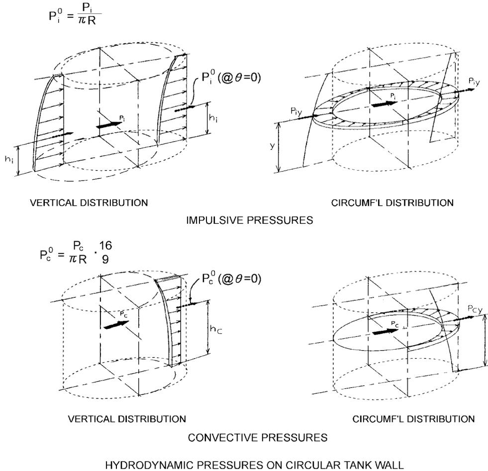
Fig. 5 Dimensions and hydrodynamic pressures on circular tank wall
