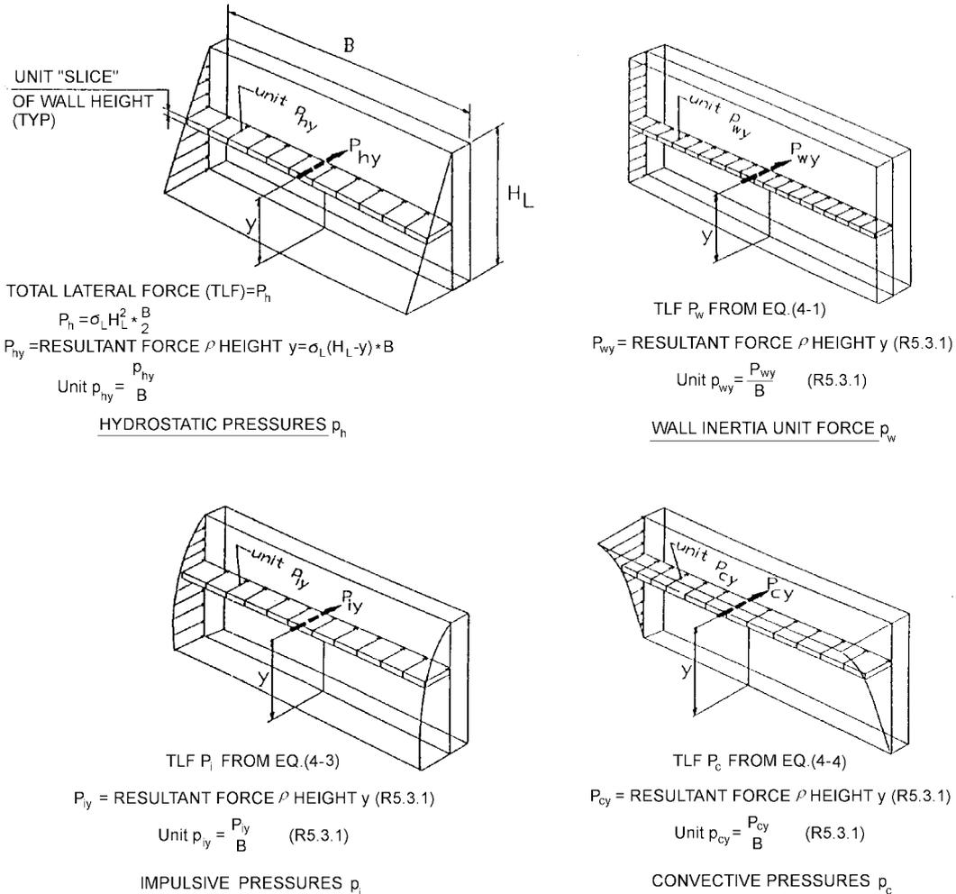
Fig. 4 Distribution of hydrostatic and hydrodynamic pressures and inertia forces
