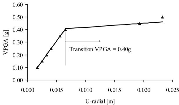
Fig. 9 VPGA vs. Displacement curve for a node in the cylinder; Tank C,  $\omega = 38.596$  rad/s.
