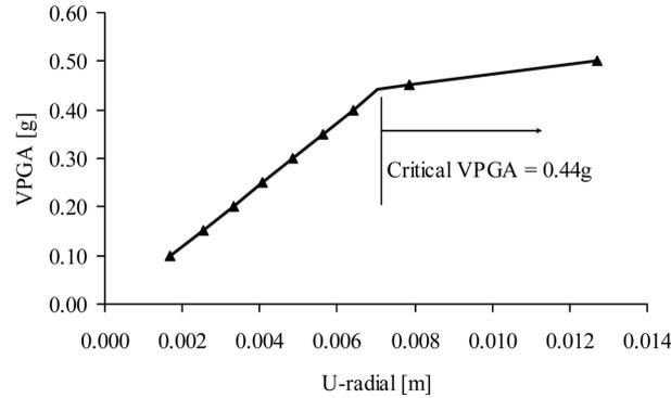
Fig. 4 VPGA versus Displacement curve for a node in the cylinder; Tank A,  $\omega = 38.601$  rad/s.
