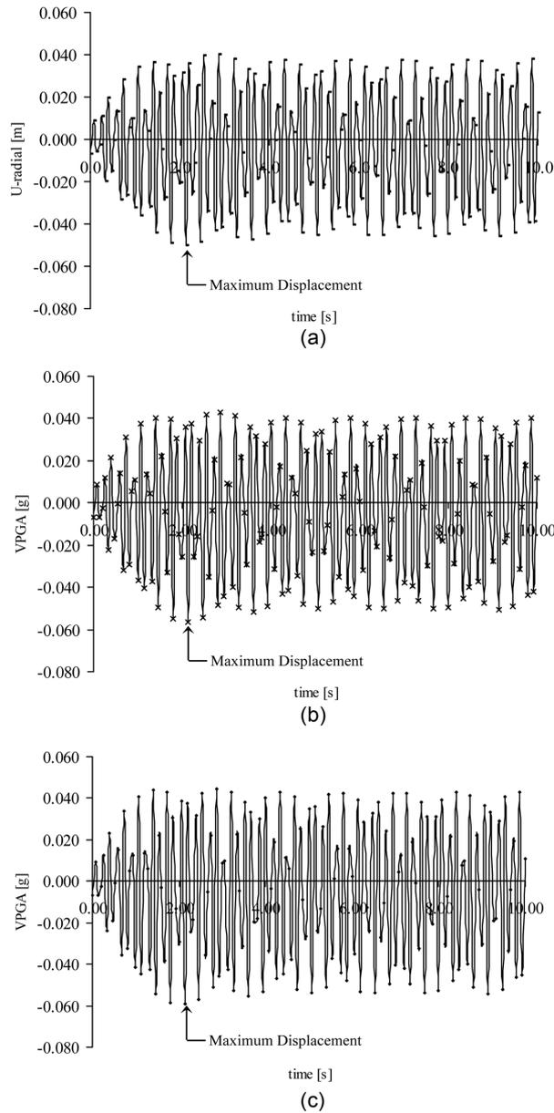
Fig. 6 Time histories for a node in the roof of Tank A;  $\omega = 38.601$  rad/s; (a) VPGA = 0.40 g, (b) VPGA = 0.45 g, (c) VPGA = 0.50 g.
