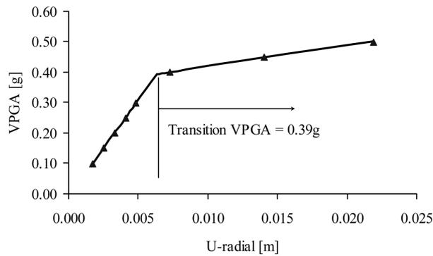
Fig. 8 VPGA vs. peak displacement curve for a node in the cylinder; Tank B,  $\omega = 38.638$  rad/s.
