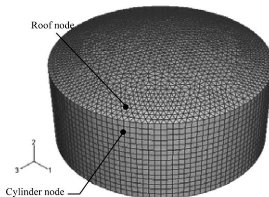
Fig. 2 Localization of nodes in the cylinder and in the roof used to investigate dynamic response.
