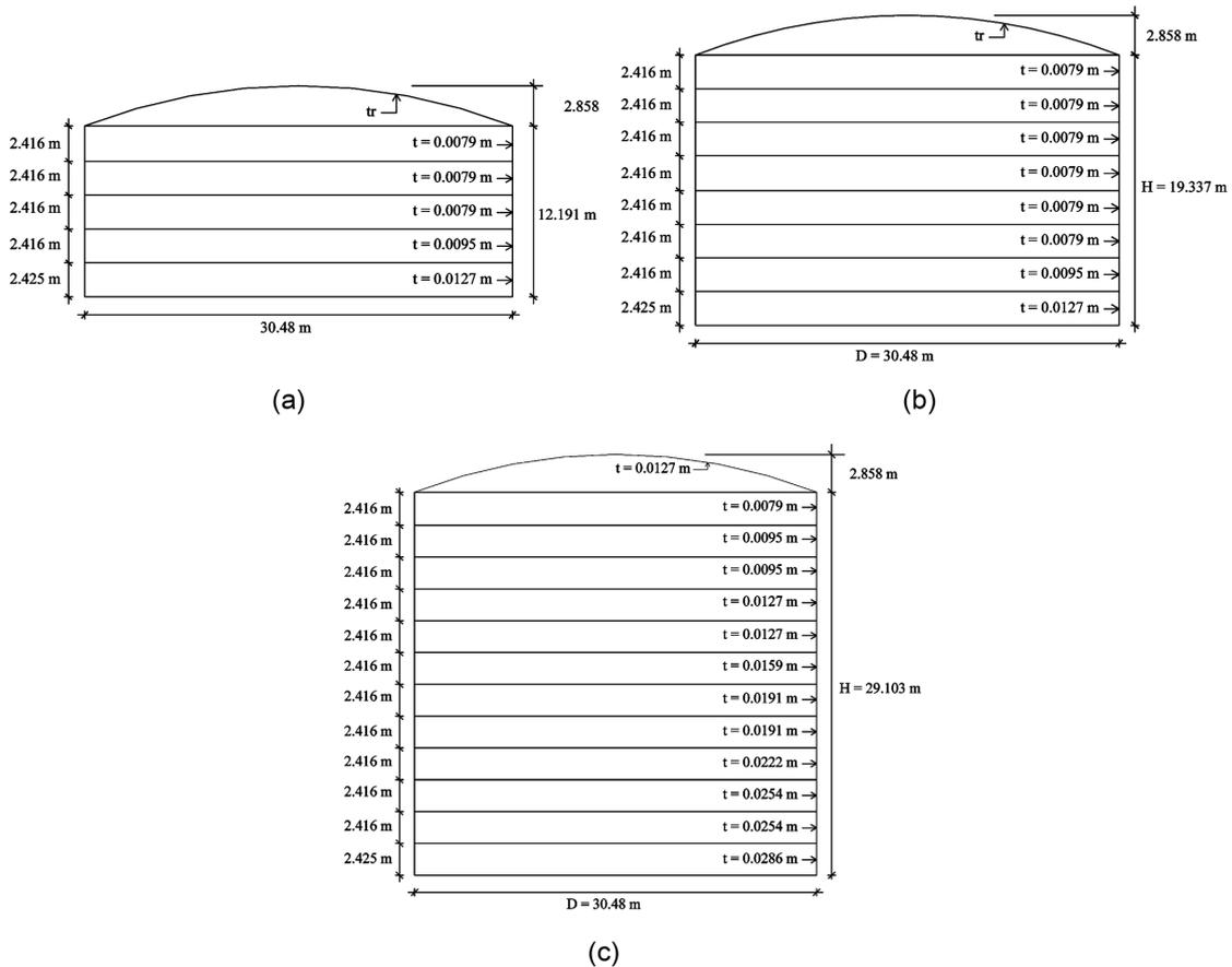
Fig. 1 Self-supported dome roof tanks. (a)  $H/D = 0.40$ ; (b)  $H/D = 0.63$ ; (c)  $H/D = 0.95$ ; roof thickness,  $tr = 0.0127$  m.
