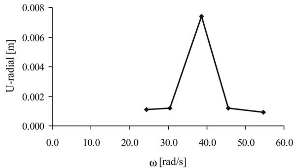
Fig. 11 Variation of maximum radial displacement  $U_{\text{-radial}}$  in the cylinder of Tank A with base motion frequency
