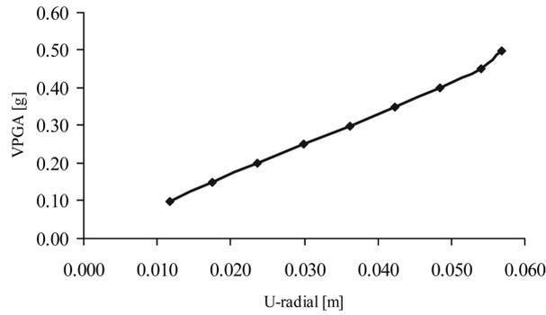
Fig. 7 VPGA versus peak displacement curve for a node in the roof; Tank A,  $\omega = 38.601$  rad/s.
