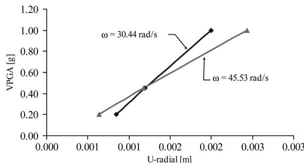
Fig. 10 VPGA versus Displacement curve for a node in the cylinder of Tank A. for case 2 ( $\omega = 30.44$  rad/s) and case 3 ( $\omega = 45.53$  rad/s).
