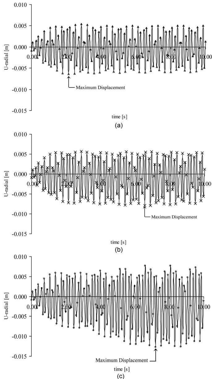
Fig. 3 Time histories for a node in the cylinder of Tank A;  $\omega = 38.601 \text{ rad/s}$ ; (a) VPGA = 0.40 g, (b) VPGA = 0.45 g, (c) VPGA = 0.50 g.
