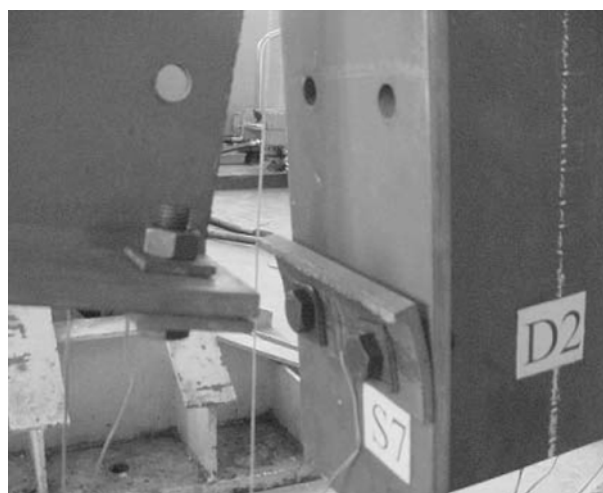
Fig. 2 Photographic view of plastic hinge line and failure pattern
