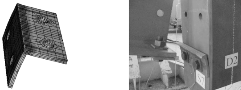
Tearing of seat angle
