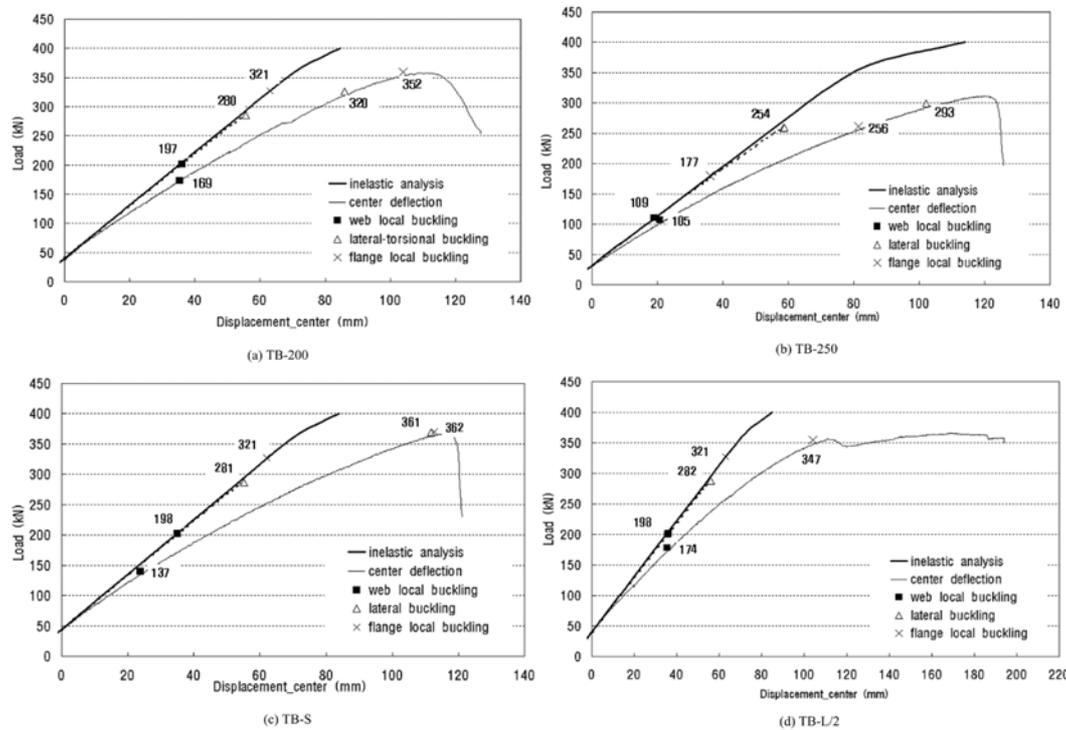
Fig. 14 Load-Displacement comparison between test and analysis
