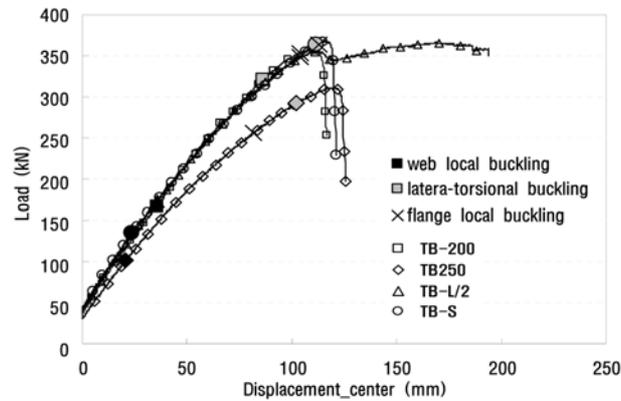
Fig. 6 Load-displacement relationship
