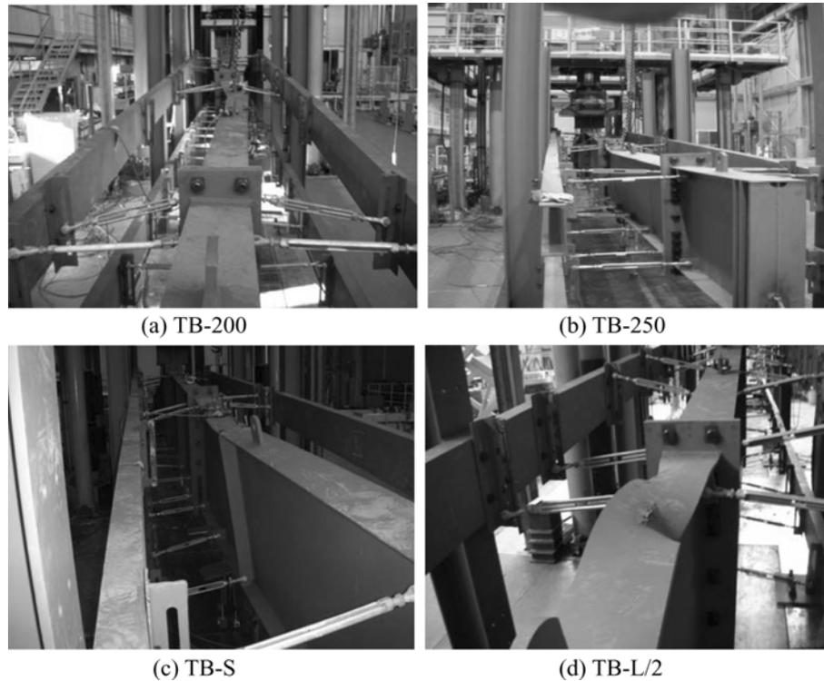
Fig. 8 Buckling shape
