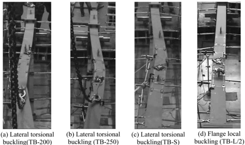
Fig. 7 Final failure mode
