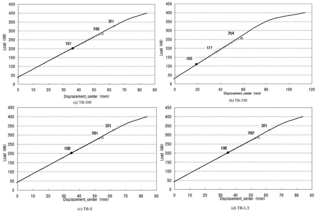
Fig. 11 Load-displacement relation and collapse mechanism of non-linear analysis
