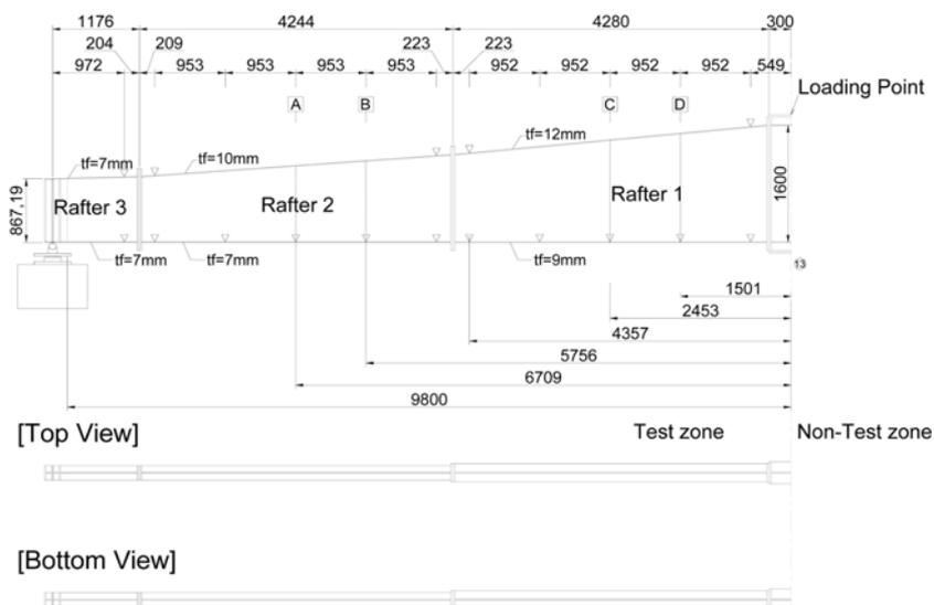
Fig. 2 Dimensions and layout of full scale test specimens
