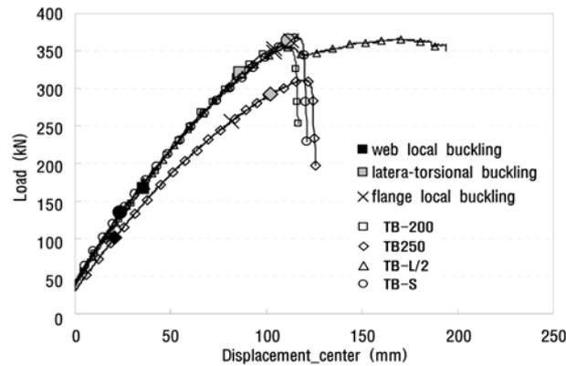
Fig. 6 Load-displacement relationship
