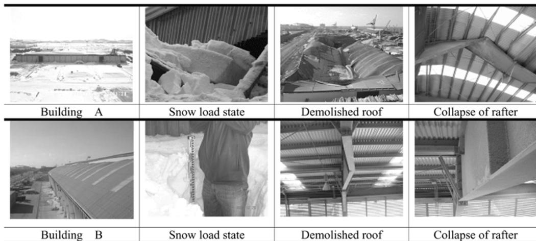
Fig. 1. Warehouse building collapse
