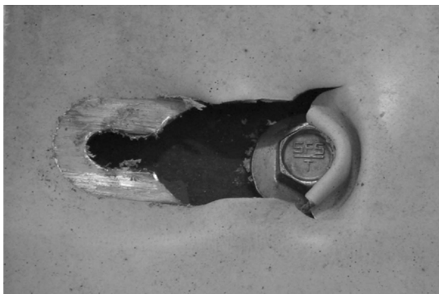
Fig. 15 The collapse mode of bolted connection at 200°C, bolt SD8-H15-5,5×25 without washer
