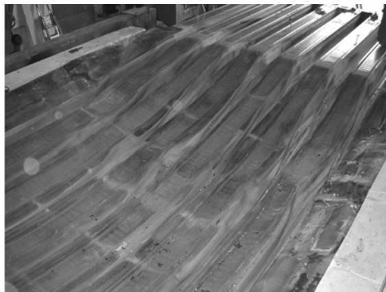
Fig. 4 Fire resistance test F2, the specimen after the test
