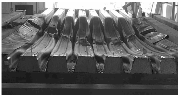
Fig. 5 Fire resistance test F2, the specimen after the test
