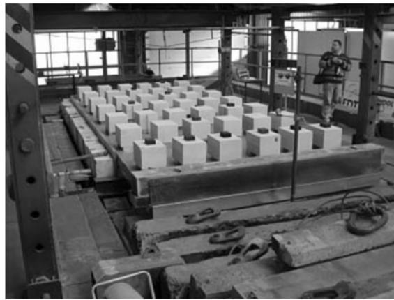
Fig. 2 Fire resistance test C3, load introduced by lightweight concrete blocks
