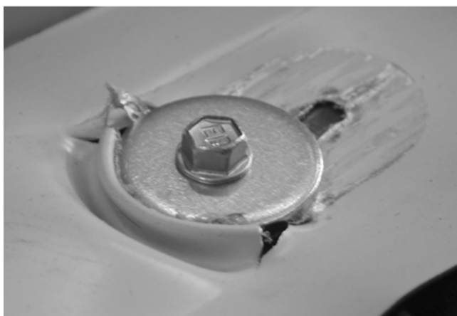
Fig. 14 The collapse mode of bolted connection at 200°C, bolt E-VS BOHR 5-5,5×38 with steel washer Ø29 mm
