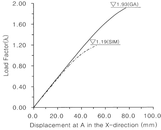
Fig. 10 Load-displacement of space two-story frame
