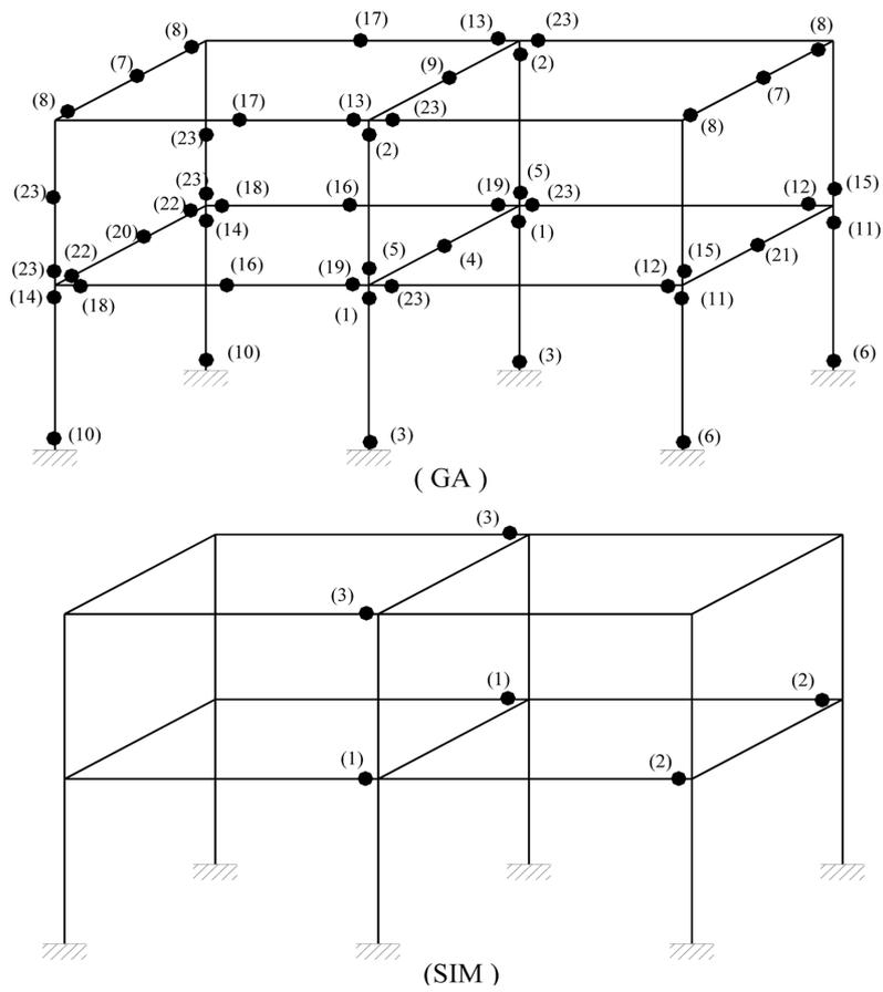
Fig. 11 Sequences of the formation of plastic hinges in the space two-story frame
