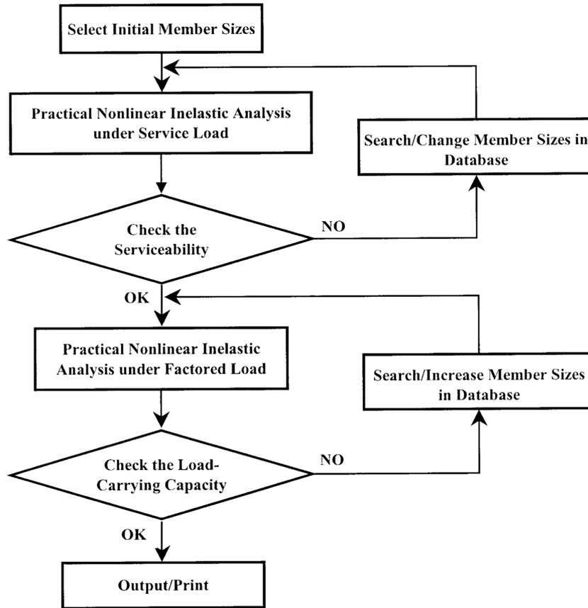
Fig. 3 Optimal design procedure using section increment method in cooperation with nonlinear inelastic analysis
