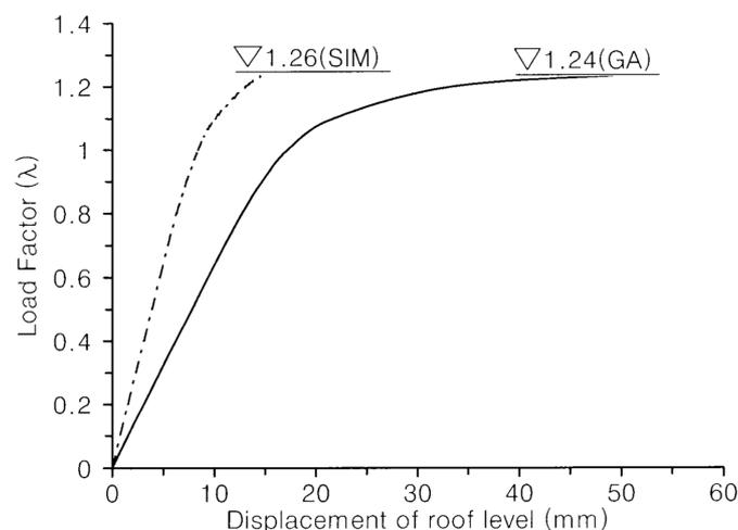
Fig. 6 Load-displacement of planar portal frame
