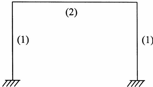
Fig. 5. Group of section types of planar portal frame
