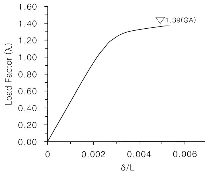
Fig. 14 Load-displacement of 3-D steel arch bridge at midspan
