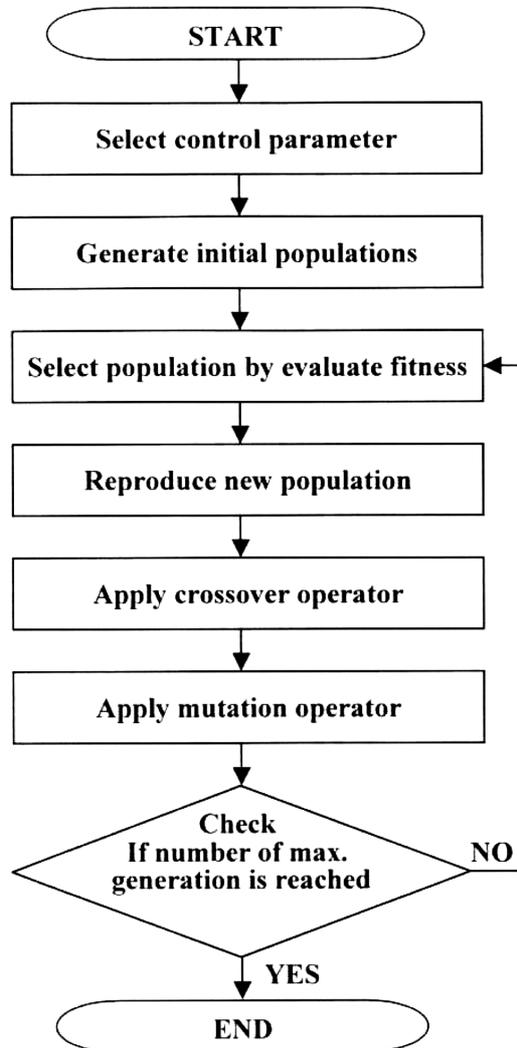
Fig. 1 Procedure of genetic algorithm
