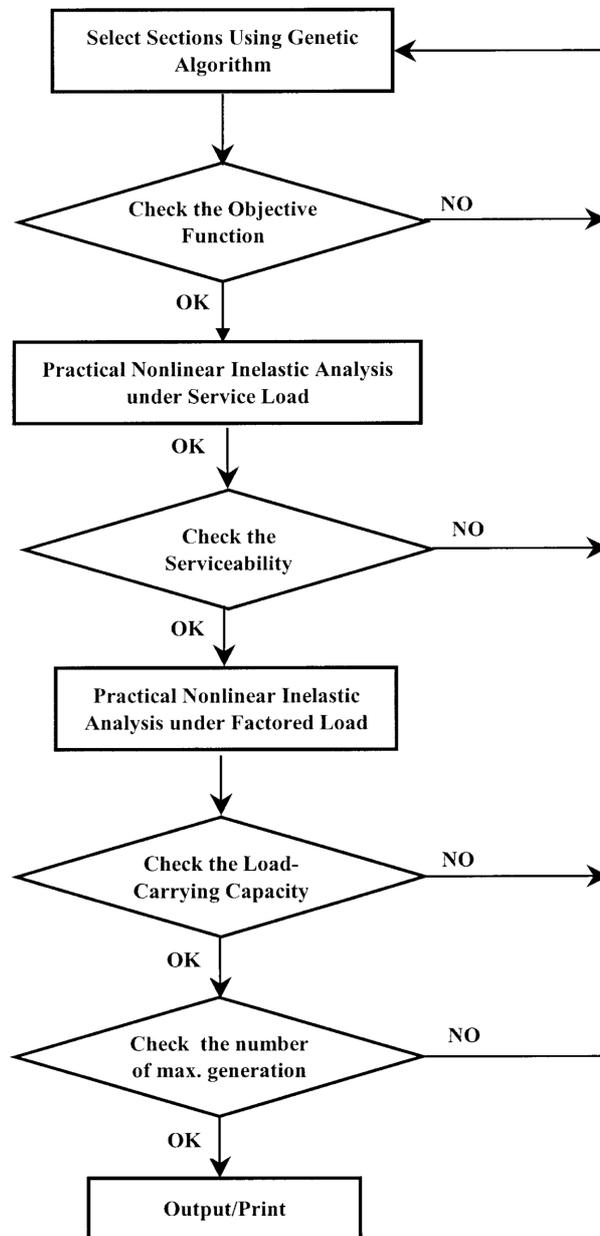
Fig. 2 Optimal design procedure using genetic algorithm in cooperated with nonlinear inelastic analysis
