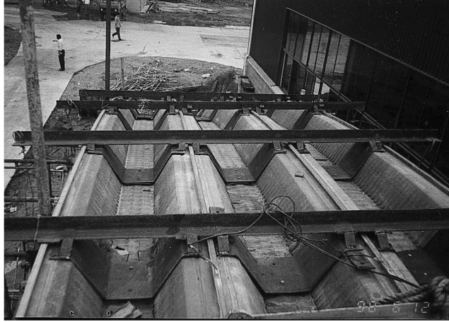
Fig. 10 Loading method and set of 18 m span samples
