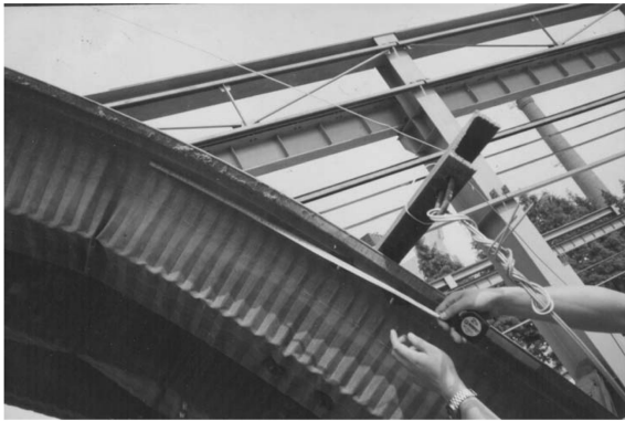
Fig. 24 Local buckle of bottom flange of 18 m span sample
