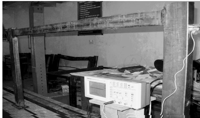
(a) Measurement of the fundamental mode of translational vibration
