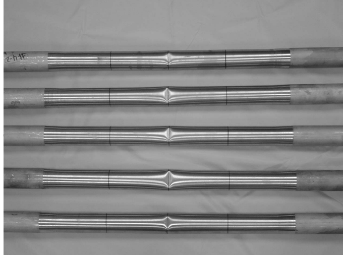
Fig. 11 A picture of the local buckling of the 316L stainless steel tubes subjected to cyclic bending
