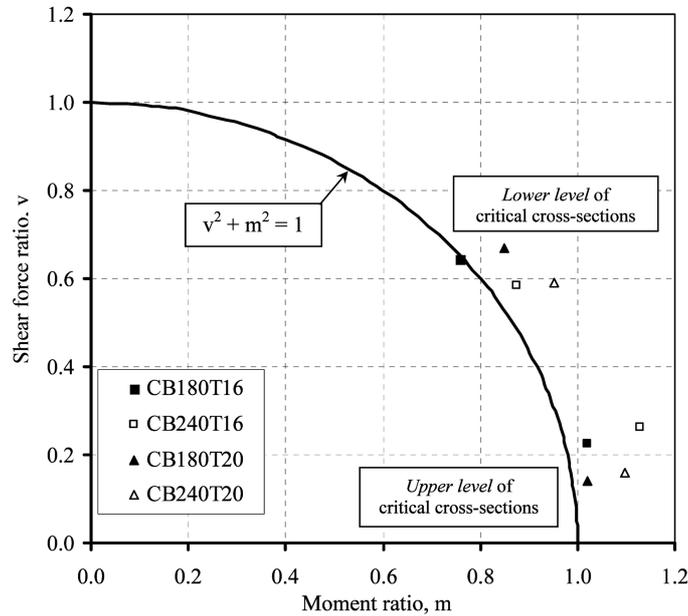
Fig. 8 Interaction curve for combined bending and shear
