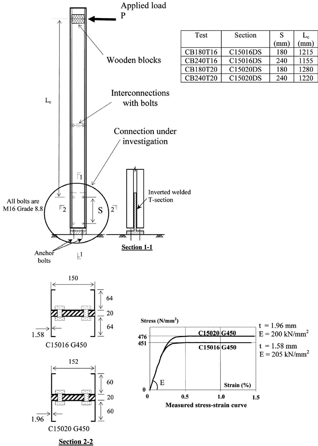
Fig. 1 Cold-formed steel column bases
