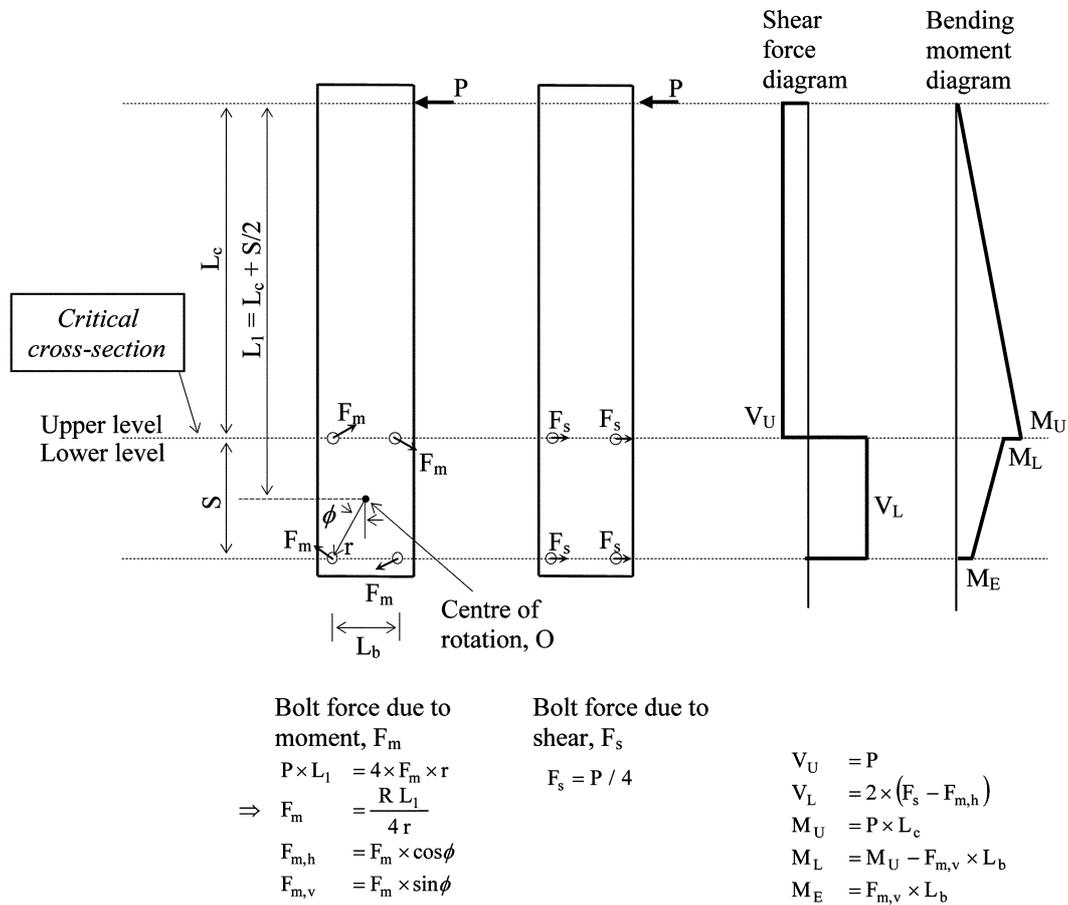
Fig. 7 Proposed design and analysis method
