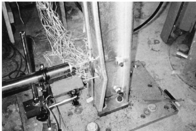
Fig. 2 Section failure at the critical cross-section under combined bending and shear
