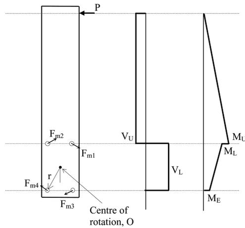
For structural adequacy of the column base connections, both the applied shear forces and the applied moments at the critical cross-sections should be checked against their respective section capacities as follows:
