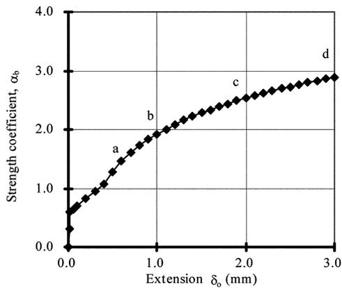
Normalized bearing deformation curve
