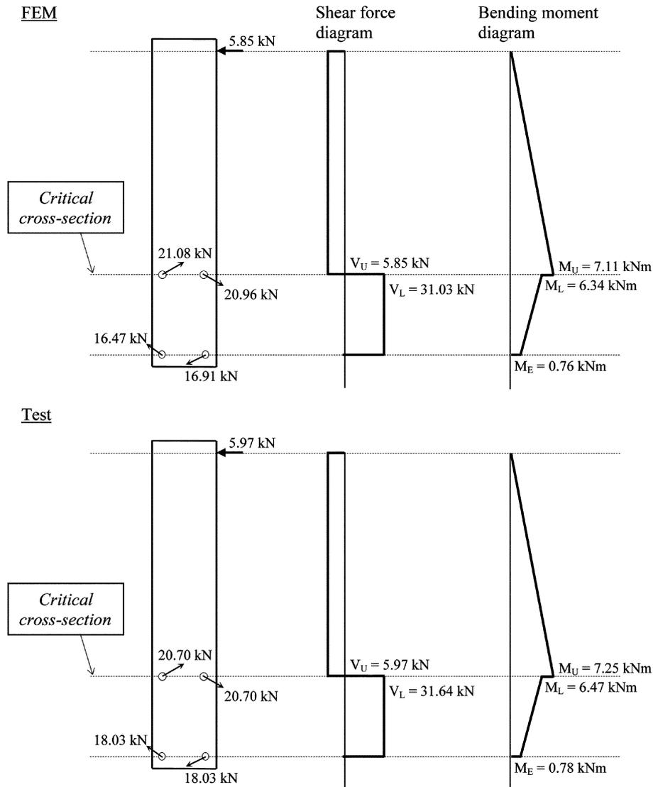
Fig. 6 Internal force distribution of Test CB180T16
