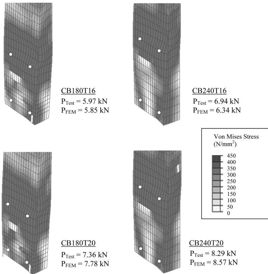
Fig. 5 Critical cross-sections of column base connections
