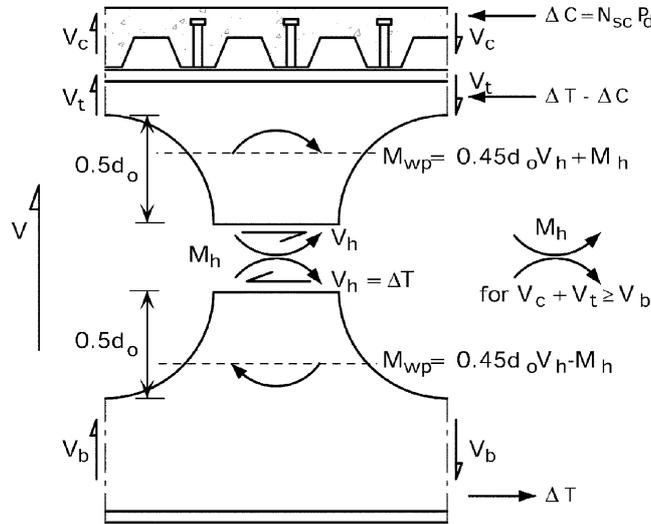
Fig. 4 Web-post moment model in cellular beams
