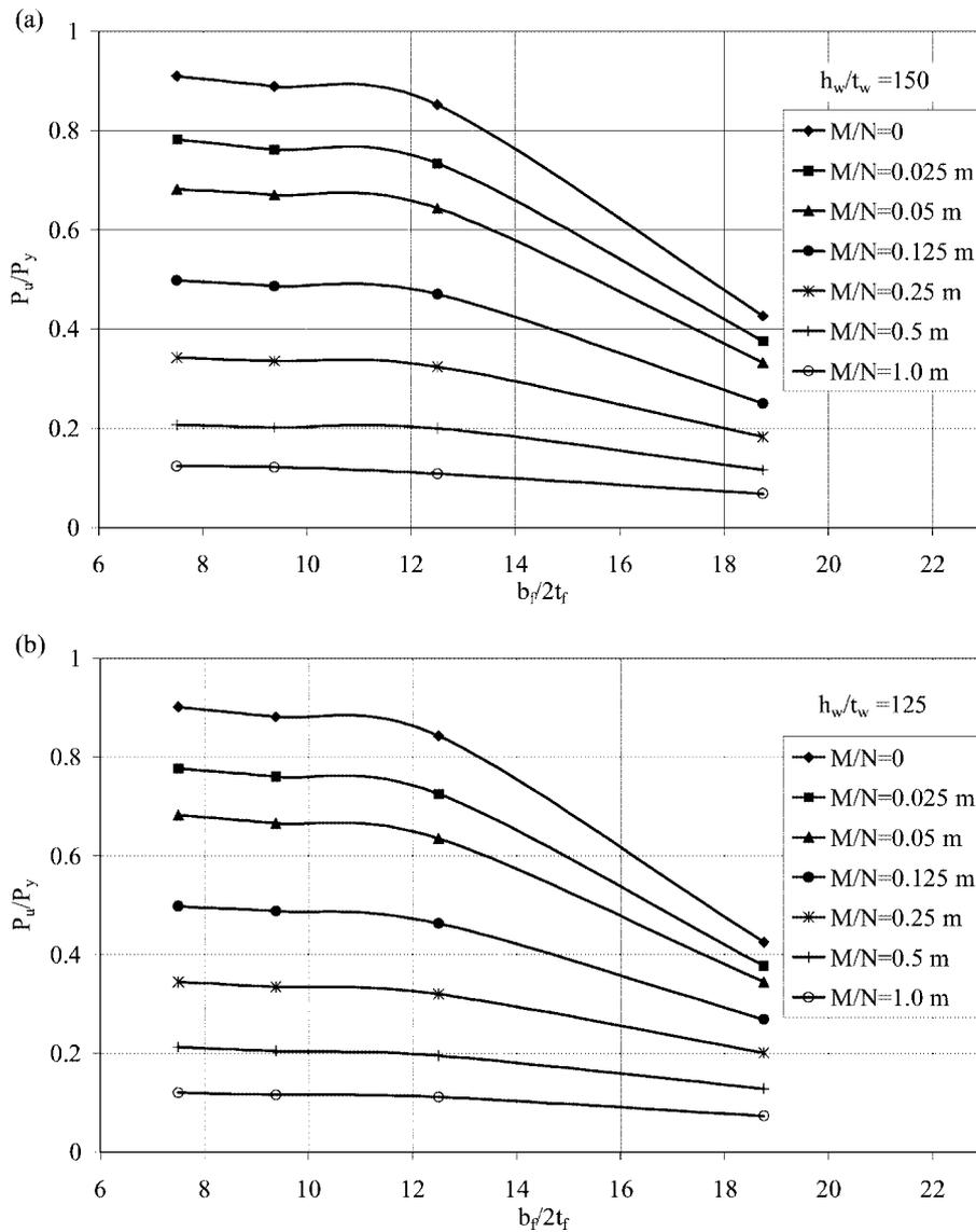
Fig. 6 Effect of  $b_f/2t_f$  on the strength of the analyzed beam-columns
