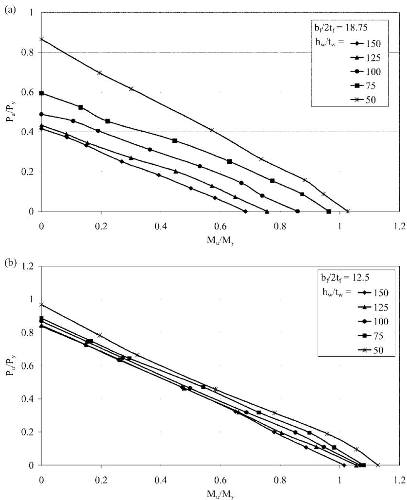
Fig. 2 Interaction diagrams for the numerically analyzed beam-columns
