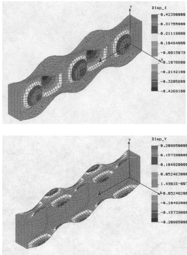
Fig. 3 Interactive local flange and web buckling mode of beam columns with  $b_f/2t_f=18.75$  and  $h_w/t_w=150$ : contour lines for the displacement in the X-direction (above) and in the Y-direction (below)
