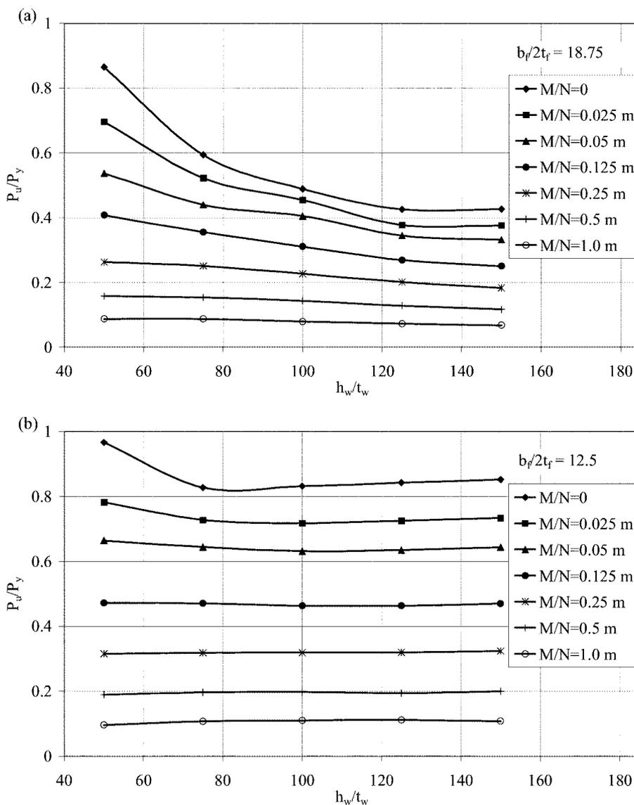
Fig. 5 Effect of  $h_w/t_w$  on the strength of the analyzed beam-columns
