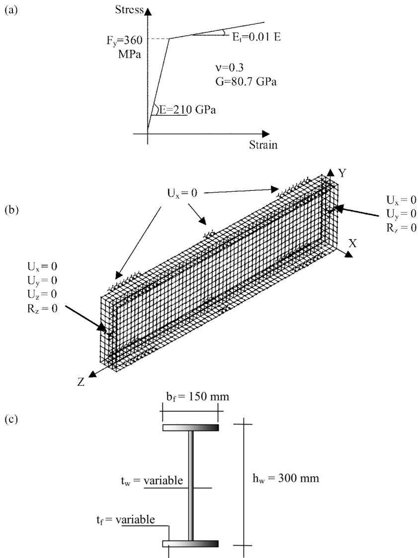
Fig. 1 Material and geometric properties of the analyzed beam-columns: (a) Conceptual uniaxial stress-strain of the steel; (b) Finite element mesh adopted in the analysis; (c) Cross-section of the analyzed beam column
