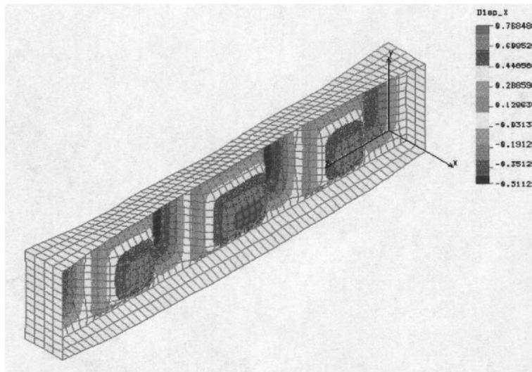
Fig. 4 Local web buckling mode of beam columns with  $b_f/2t_f=7.5$  and  $h_w/t_w=150$ : contour lines for the displacement in the X-direction
