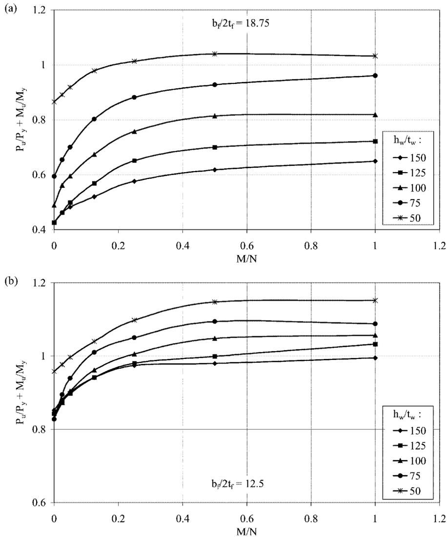
Fig. 7 Effect of  $M/N$  on the strength of the analyzed beam-columns
