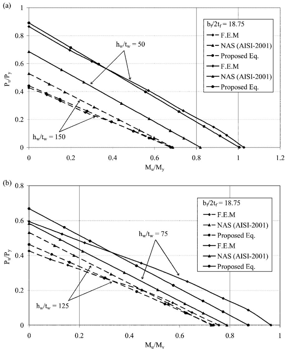
Fig. 8 A typical comparison between beam-column strength predicted based on the NAS (AISI-2001), the numerical analysis and the proposed design method
