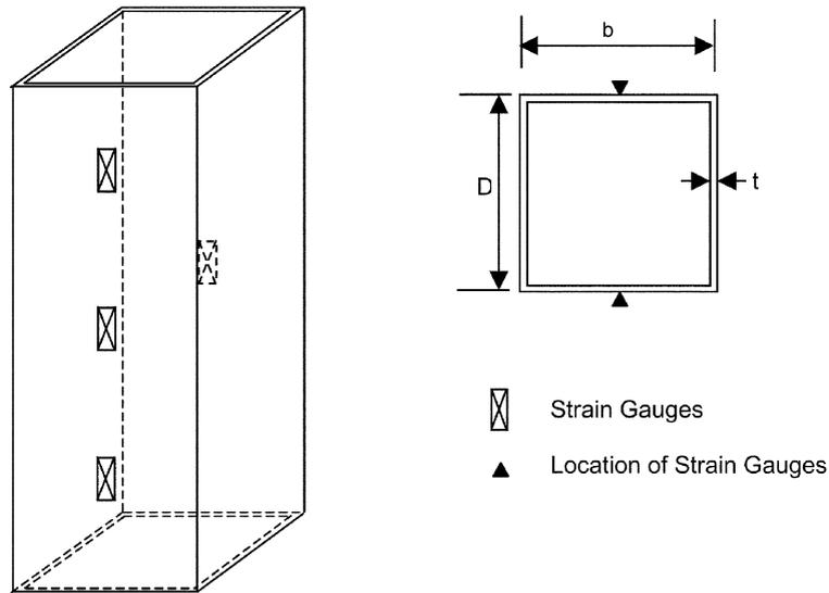
Fig. 4 Strain gauges location
