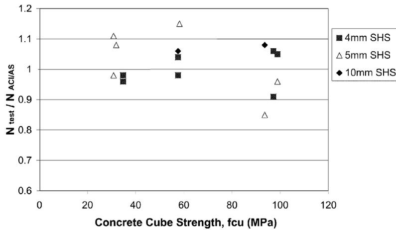
Fig. 13  $N_{test} / N_{ACI/AS}$  vs concrete cube strength
