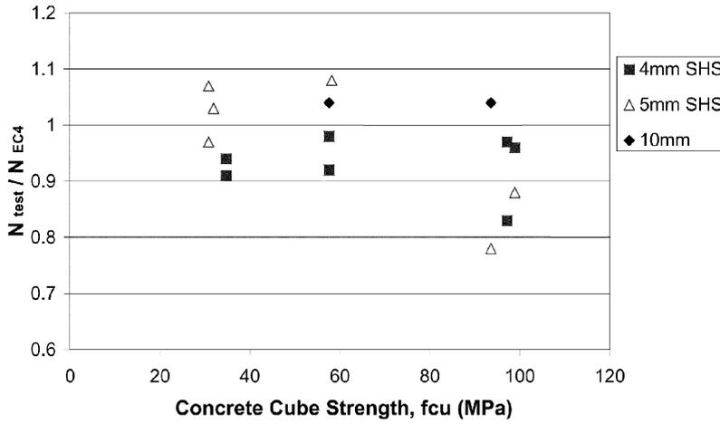
Fig. 11  $N_{test} / N_{EC4}$  vs concrete cube strength
