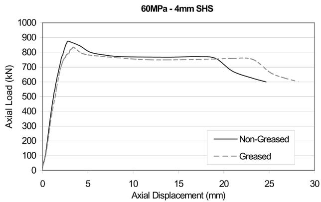
Fig. 8 Axial load-displacement, Non-Greased and Greased, 60 MPa concrete
