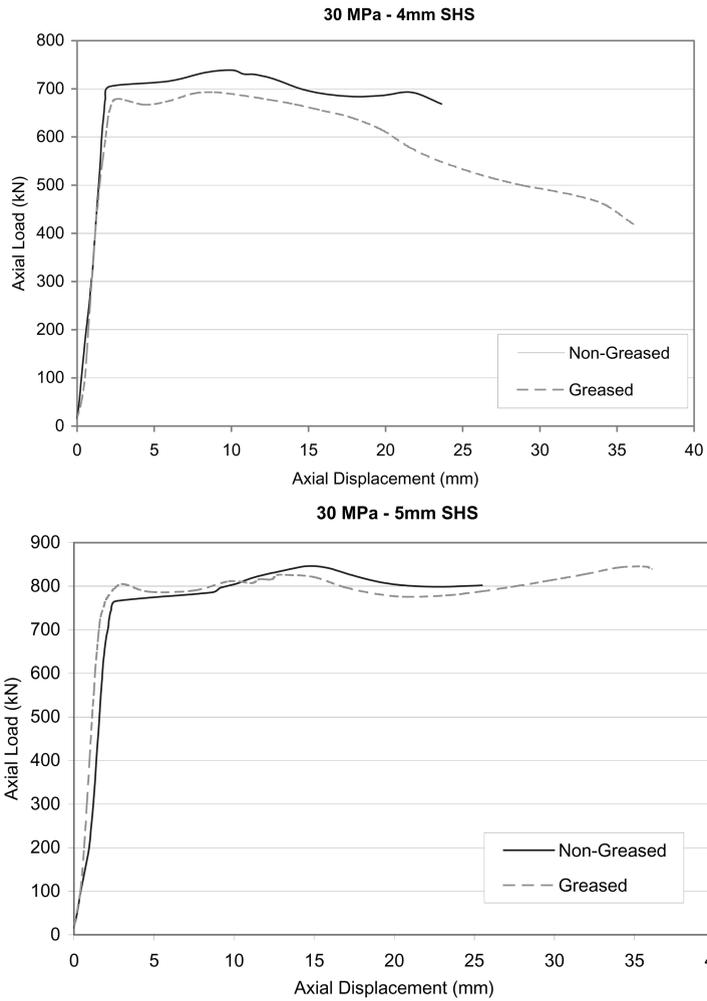
Fig. 7 Axial load-displacement, Non-Greased and Greased, 30 MPa concrete
