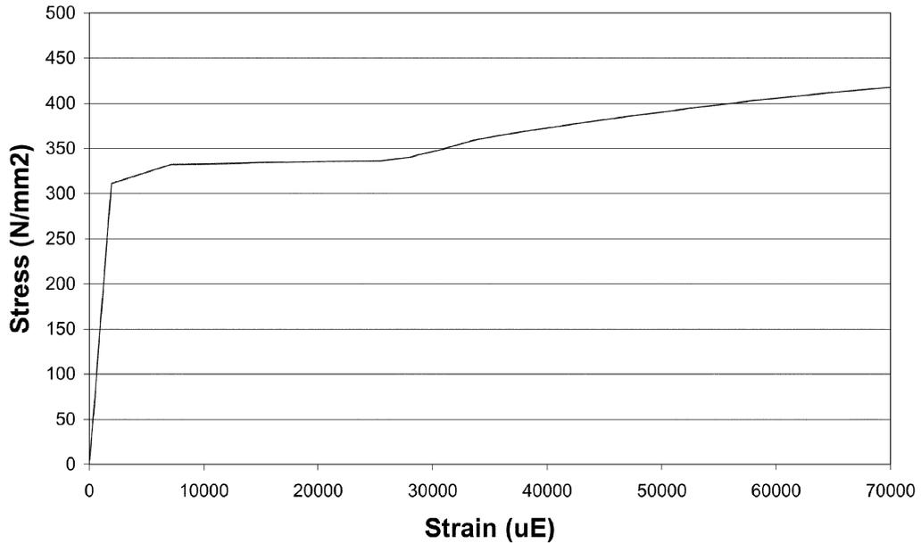
Fig. 3 Stress vs strain curve of 4 mm SHS
