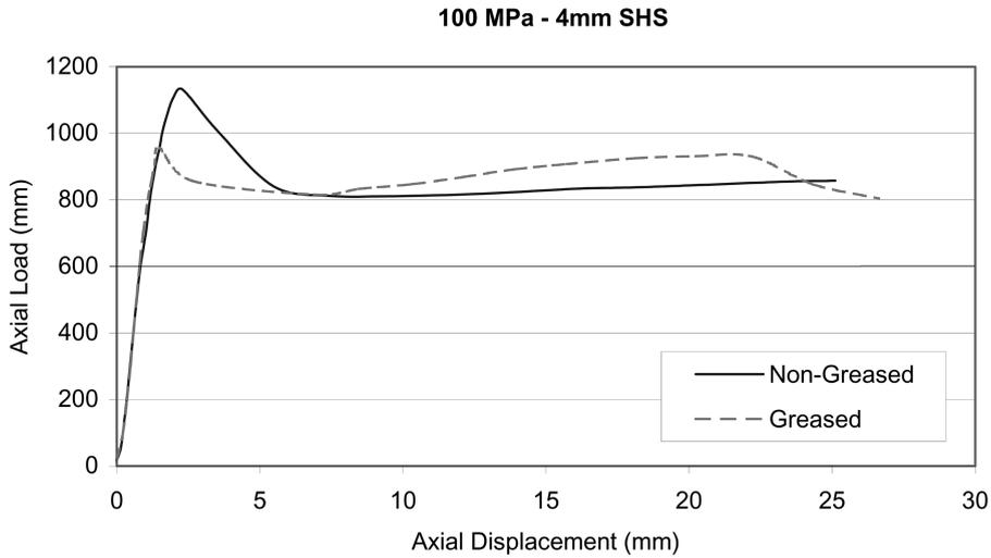
Fig. 9 Axial load-displacement, Non-Greased and Greased, 100 MPa concrete
