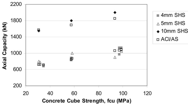
Fig. 12 Comparison of ACI and AS with experimental results
