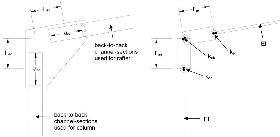
Fig. 12. Beam idealisation of eaves joint
