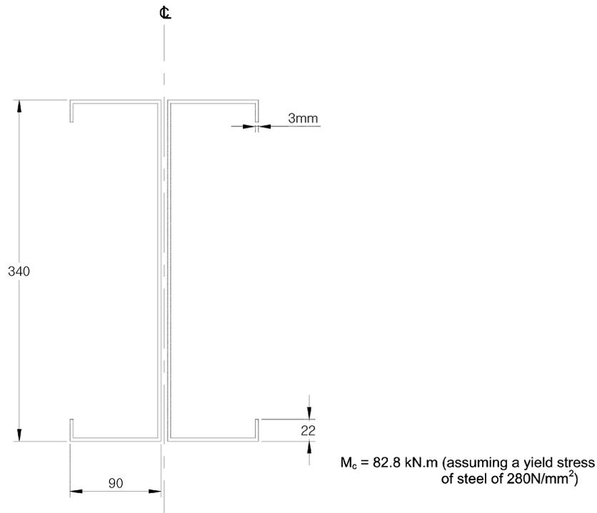
Fig. 6 Dimensions of back-to-back channel-section used for column and rafter members
