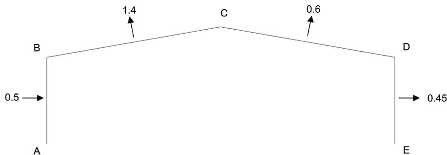
Fig. 7 Coefficients of wind pressure for wind load combination 1 (WLC1)
