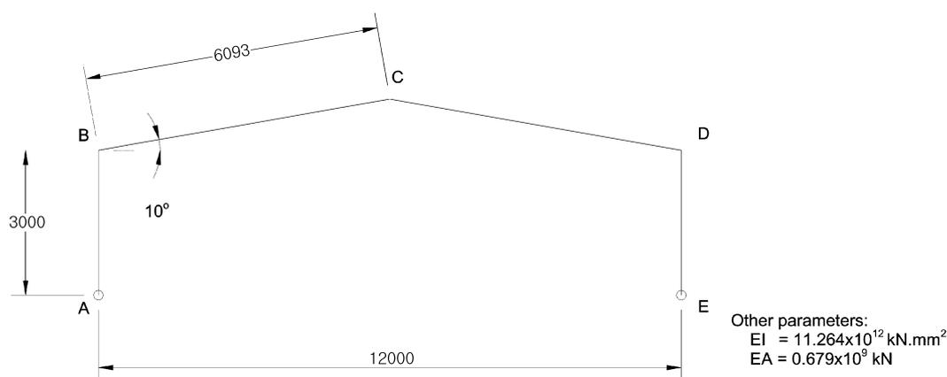
Fig. 5 Details of standard portal frame used in study
