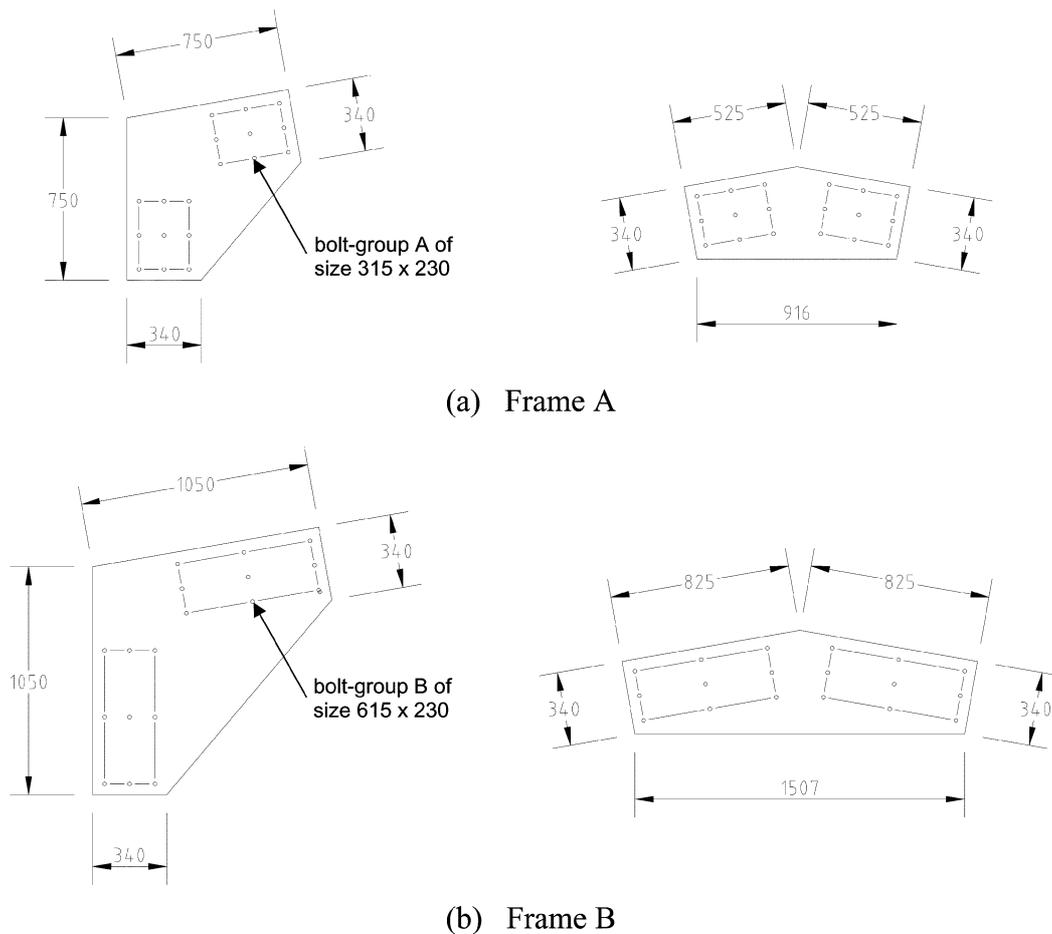
Fig. 11 Details of bolt-groups and corresponding sizes of eaves and apex brackets
