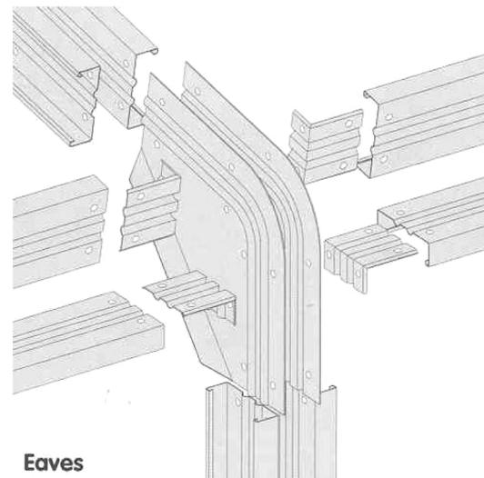
Fig. 2 Details of the eaves joint of the Swagebeam (courtesy of Ayrshire)
