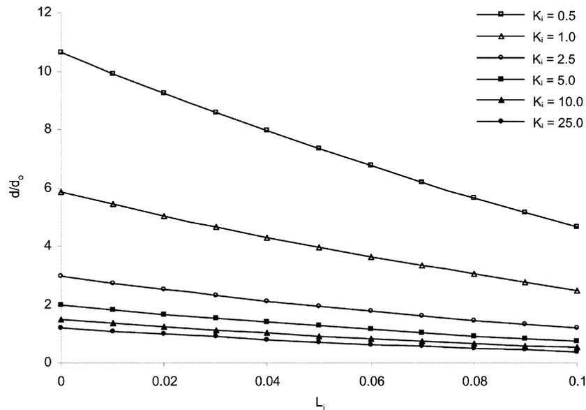
Fig. 17 Variation of critical apex deflection against connection-length for various values of joint rotational stiffness for frame of aspect ratio  $L_f/h_f = 3$  under vertical load
