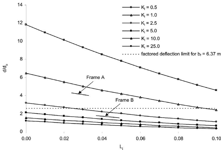
Fig. 16 Variation of apex deflection against connection-length for various values of joint rotational stiffness of joint for standard frame under wind load combination 1 (WLC1)
