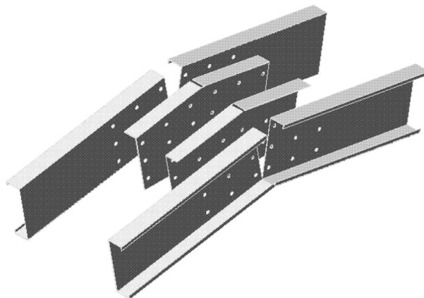
Fig. 4 Details of the proposed arrangement for the apex joint
