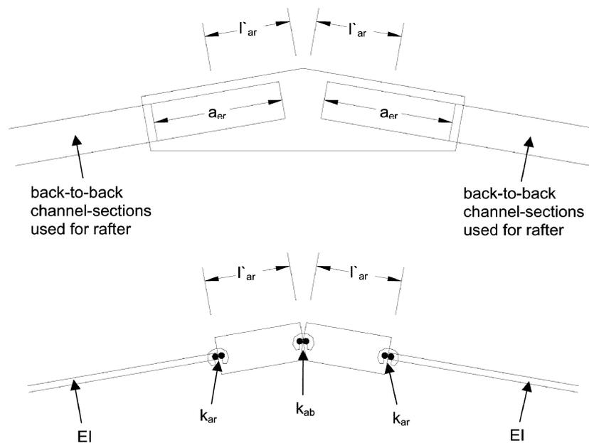
Fig. 13 Beam idealisation of apex joint
