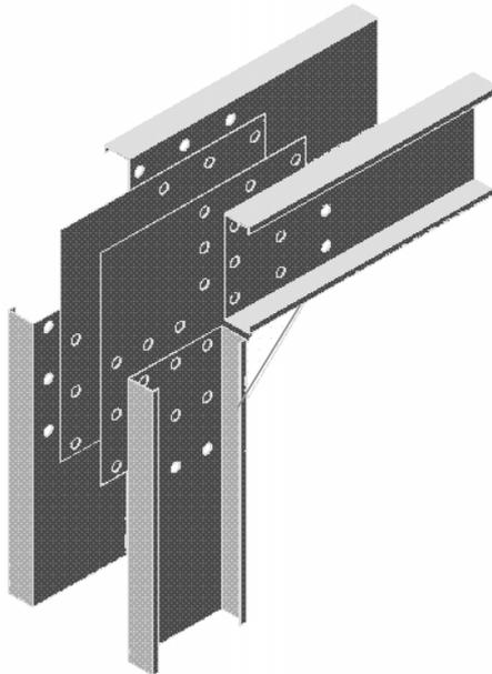
Fig. 3 Details of the proposed arrangement for the eaves joint
