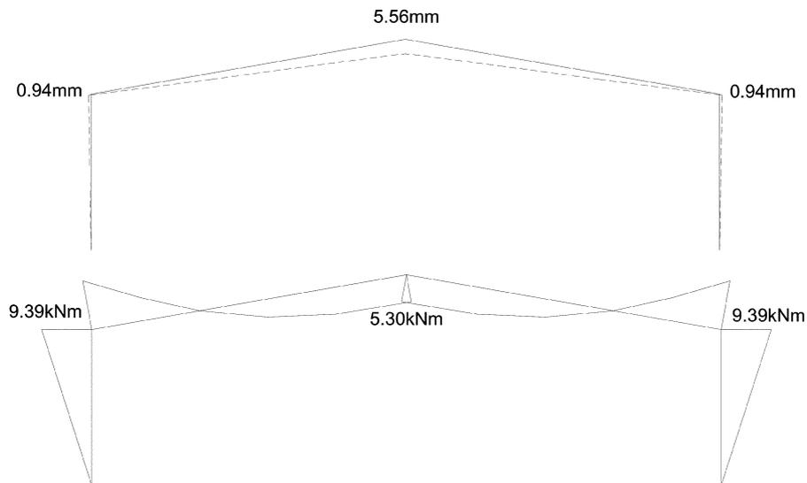
Fig. 9 Deflected shape and bending moment diagram of rigid-jointed portal frame under 1 kN/m uniformly distributed vertical load
