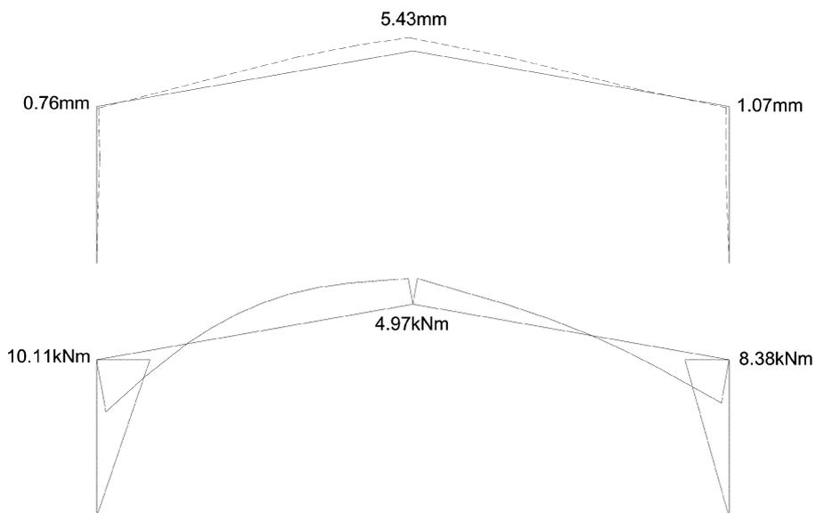
Fig. 10 Deflected shape and bending moment diagram of rigid-jointed portal frame under uniformly distributed load corresponding to the coefficients of pressure for wind load combination 1 (WLC1)
