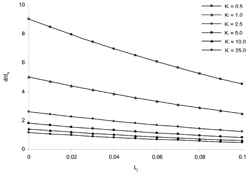
Fig. 18 Variation of critical apex deflection against connection-length for various values of joint rotational stiffness for frame of aspect ratio  $L_f/h_f = 2$  under vertical load
