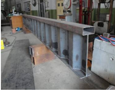
Fig. 8 Specimen of I-girder with a span of 6m and test rig
