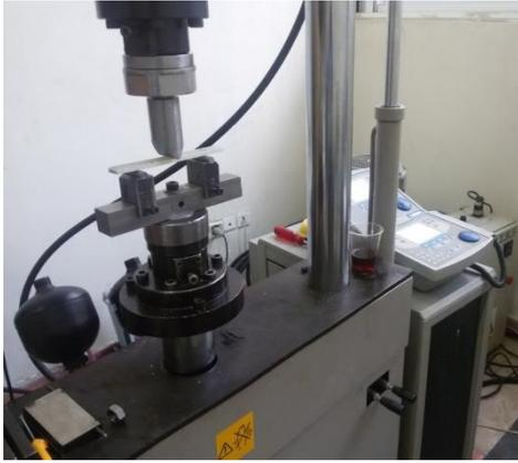
Fig. 4 The ENF test apparatus and fixture used in the experiments
