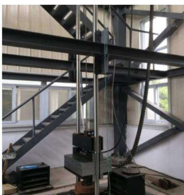
(a) Impact load test system
