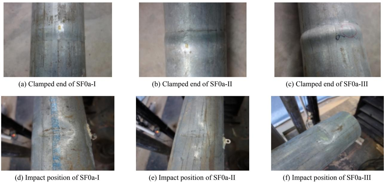
Fig. 3 Typical damage modes of steel tubes
