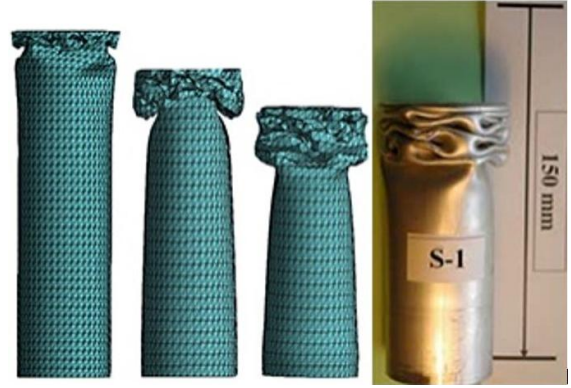
Fig. 5 Comparison of the deformed shapes between finite element method (FEM) solution and experiment (Zarei and Kröger 2006)
