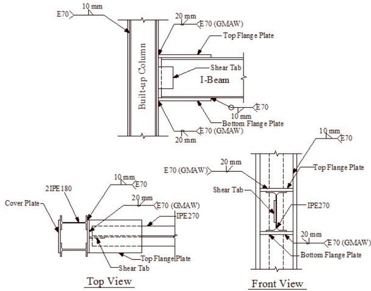
Fig. 5 Details of TMC specimen
