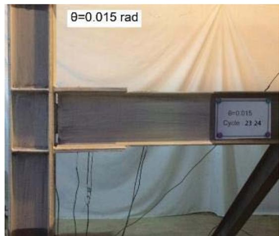
Fig. 17 Linear behavior of the MMC up to 1.5% drift angle
