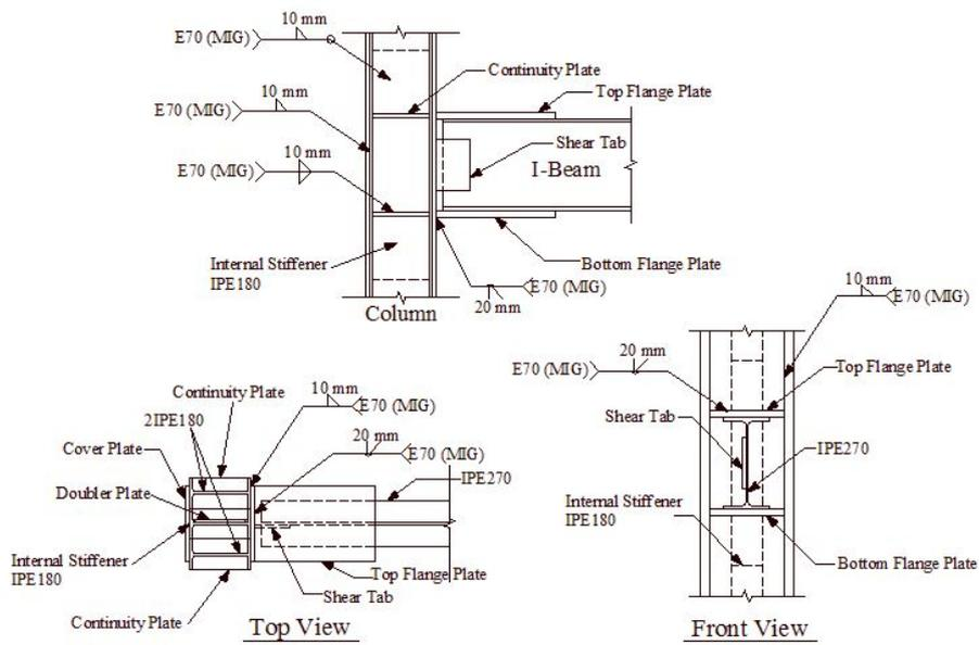
Fig. 6 Details of MMC specimen
