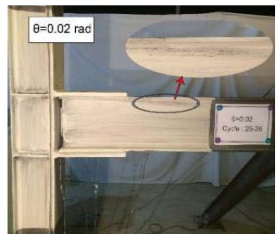
Fig. 18 Initiating yielding of the beam in the MMC at 2% drift angle
