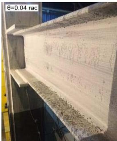
Fig. 20 Yielding of the beam in the MMC at 4% drift angle
