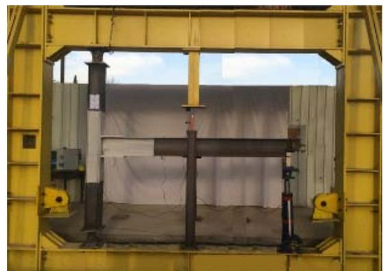
Fig. 8 Photo of test setup and loading frame
