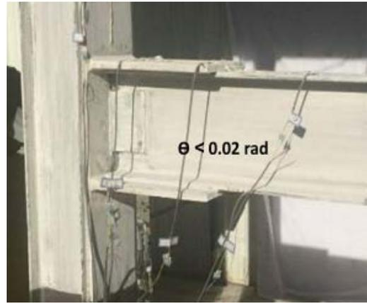
Fig. 13 Linear behavior of the TMC up to 1.5% drift angle
