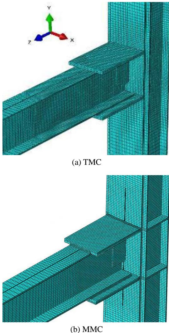
Fig. 22 3D view of the test specimens modeled in ABAQUS
