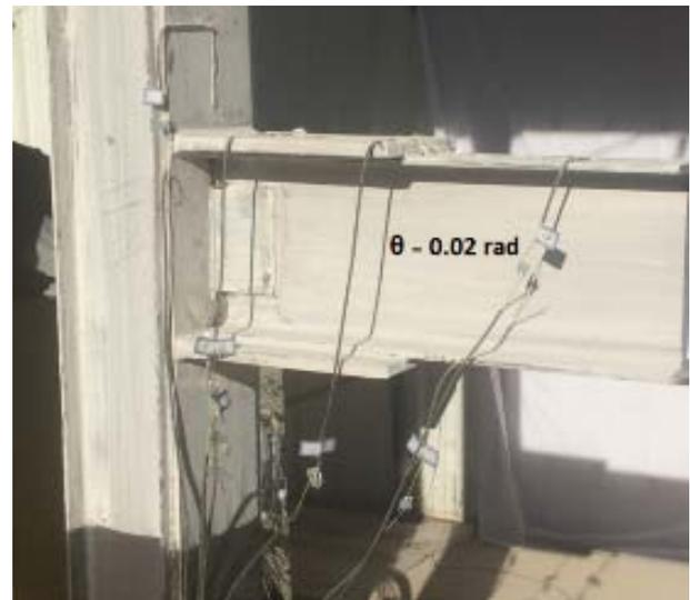
Fig. 14 Initiating nonlinear behavior of the panel zone in the TMC at 2% drift angle
