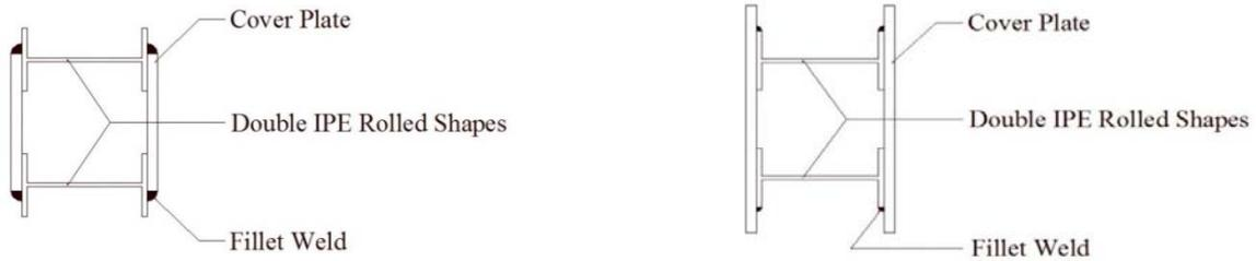
Fig. 1 Typical sections of built-up double-I columns
