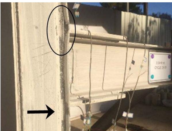
Fig. 16 Complete tearing of IPE's flange and formation of plastic zone in back of the column's flange in the TMC specimen at 4% drift angle
