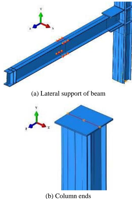
Fig. 23 Boundary conditions of the connection specimens
