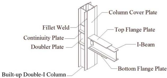
Fig. 2 WFP beam-column connection in steel intermediate MRFs with BD-I column section
