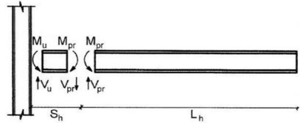
Fig. 4 Free body diagram of exterior MRF connection
