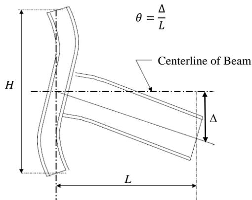
Fig. 9 Deformation of the exterior beam-column connection
