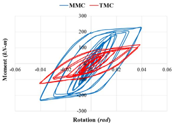
Fig. 12 Comparing hysteresis moment-rotation behavior of TMC and MMC samples
