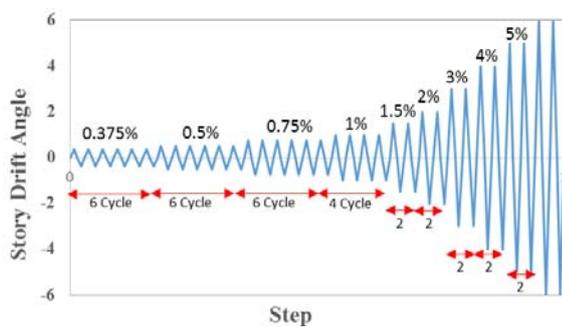
Fig. 10 Cyclic loading protocol of AISC 341
