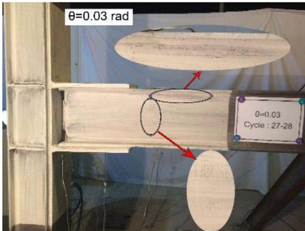
Fig. 19 Considerable nonlinear behavior in flange and web of the MMC at 3% drift angle
