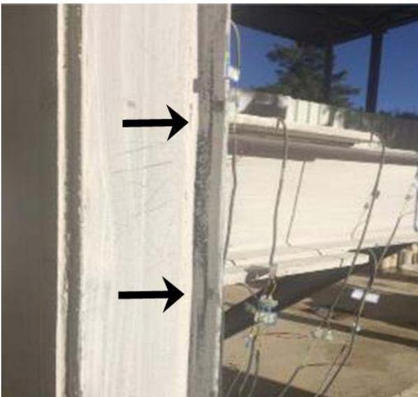
(b) Tearing in the column's flange
