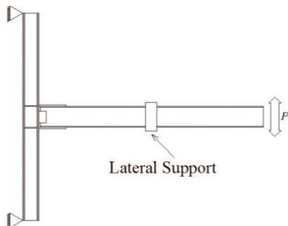
Fig. 7 Schematic diagram of exterior beam-column connection test setup
