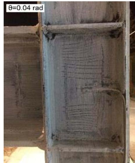
Fig. 21 Nonlinear behavior of the panel zone in the MMC at 4% drift angle
