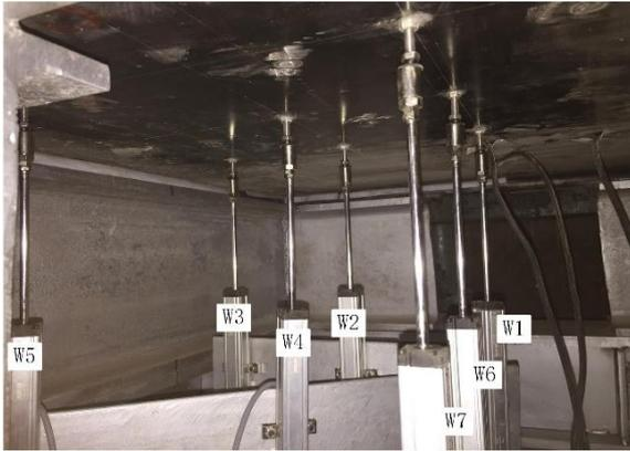
Fig. 3 Measuring points at the bottom steel faceplate
