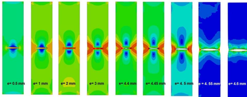
Fig. 9 The FE analysis results: Von Mises stress distribution in different elongations
