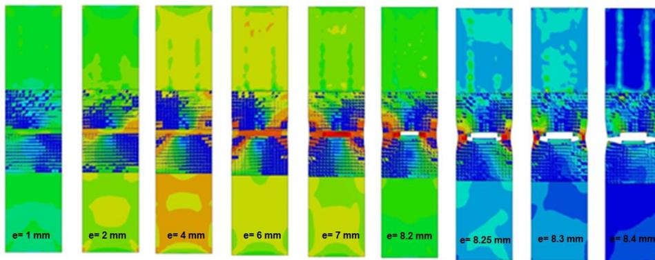
Fig. 10 The FE analysis results of specimen with adhesively bonded composite patch in different elongations
