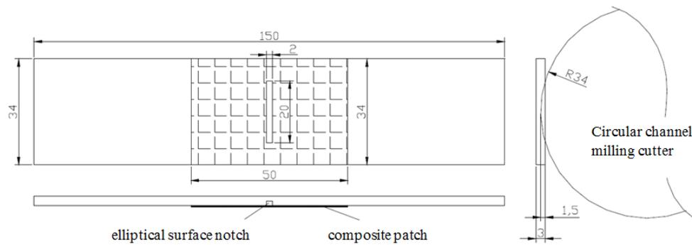
Fig. 1 Views and dimension of test specimen with elliptical surface notch and composite patch
