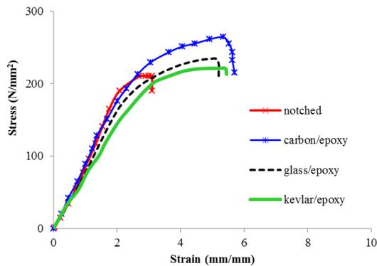
Fig. 5 The stress-strain curves of the repaired specimens
