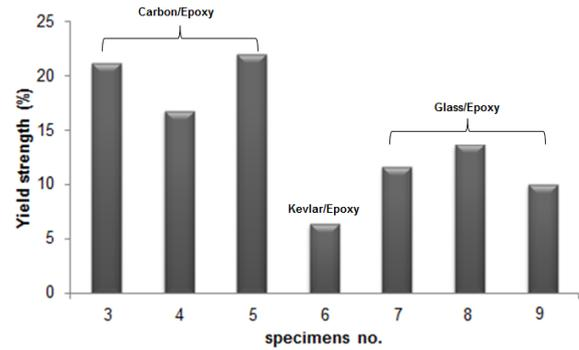
Fig. 6 The percentage increase of the tensile yield strength of repaired specimens in comparison to unrepaired specimen
