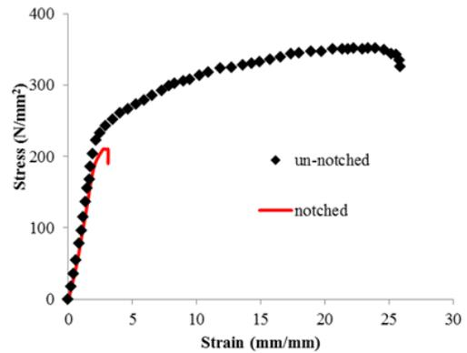
Fig. 4 The stress-strain curves of the un-notched and notched specimens
