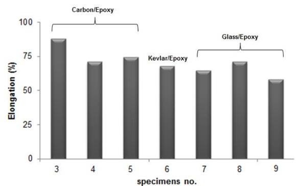
Fig. 8 The percentage increase of elongation of repaired specimens in comparison to unrepaired specimen
