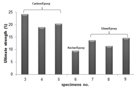
Fig. 7 The percentage increase of the ultimate tensile strength of repaired specimens in comparison to unrepaired specimen
