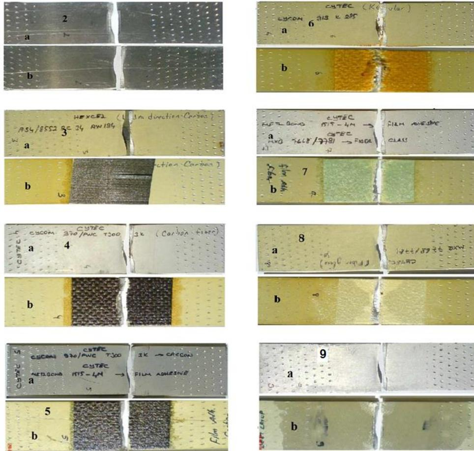
Fig. 3 (a) front views and (b) back views of specimens after tensile test
