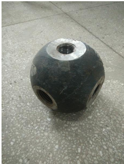
Fig. 4 Bolt sphere specimens
