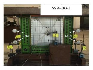
Fig. 5 Installation place of the transducers and the strain gauges in the SSW-BO-1 specimen
