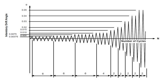
Fig. 6 Loading protocol based on SAC (FEMA, 2000)
