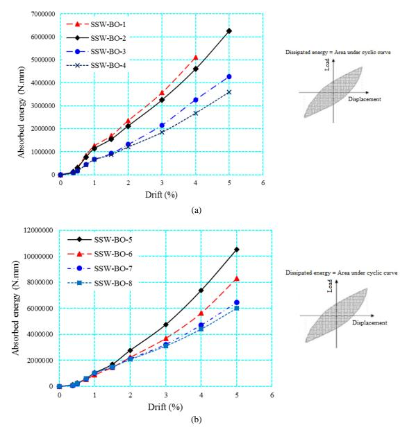
Fig. 14 The relationship curve of area of hysteretic curves versus story drift: (a) For specimens with infill plate of 0.8 mm thickness and (b) For specimens with infill plate of 1.25 mm thickness
