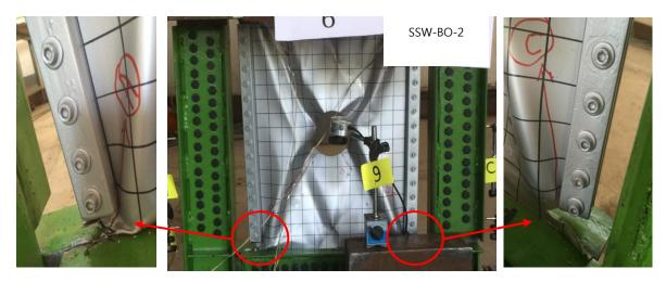
Fig. 8 Local tears at the lower corners of SSW-BO-2
