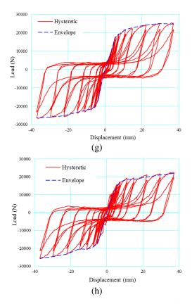
Fig. 12 Force-displacement hysteretic curve of the specimens: (a) SSW-BO-1, (b) SSW-BO-2, (c) SSW-BO-3, (d) SSW-BO-4, (e) SSW-BO-5, (f) SSW-BO-6, (g) SSW-BO-7 and (h) SSW-BO-8
