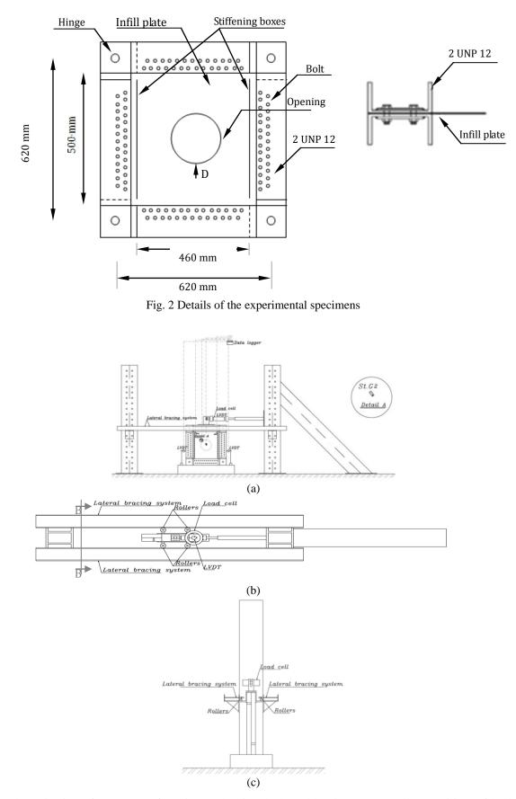
Fig. 3 Schematic view of test set-up of specimens showing the lateral bracing system, rollers, positions of load cell, LVDTs and strain gauges; (a) Front view, (b) Top view and (c) Section B-B
