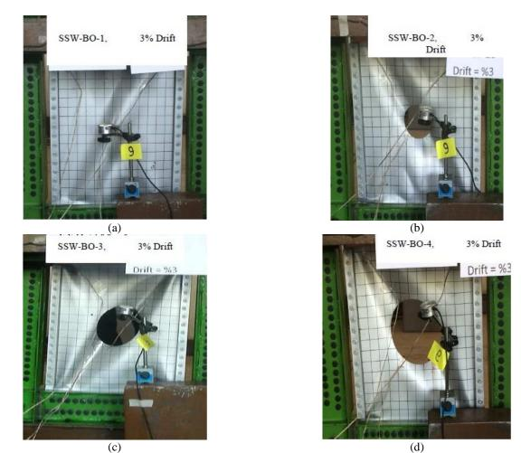
Fig. 11 Out of plane deformation at 3% drift: (a) SSW-BO-1, (b) SSW-BO-2, (c) SSW-BO-3 and (d) SSW-BO-4
