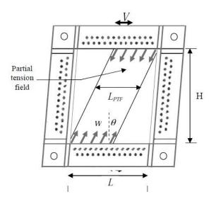
Fig. 20 Steel plate connected to frame beams only
