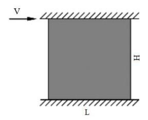
Fig. 19 Steel plate connected to frame beams only (Gue *et al.* 2011)
