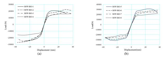
Fig. 13 The hysteresis envelope curves: (a) For specimens with infill plate of 0.8 *mm* thickness and (b) For specimens with infill plate of 1.25 mm thickness
