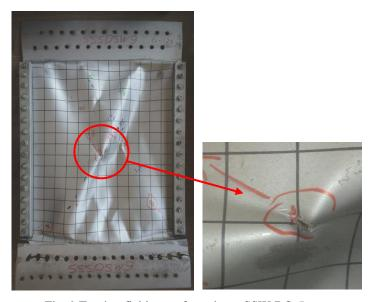
Fig. 9 Tension field tear of specimen SSW-BO-5
