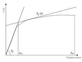
Fig. 15 Determination of yielding displacement  $\Delta_v$
