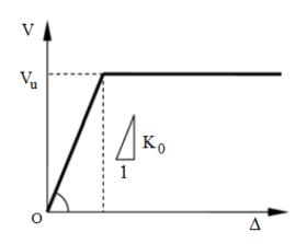
Fig. 18 Simplified model of shear forcedisplacement Skeleton curve of a steel plate (Gue *et al.* 2011)
