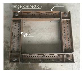
Fig. 1 Hinge type connections in boundaries at four corners
