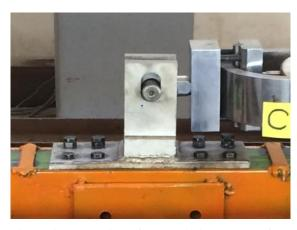
Fig. 4 Pin connection of hydraulic jack to top of the specimens
