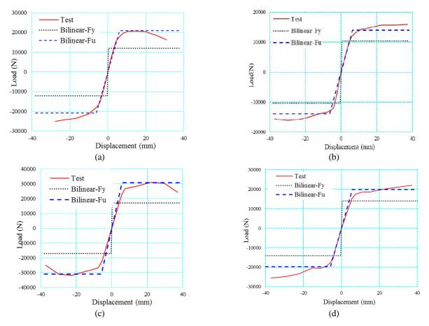
Fig. 21 Comparison of experimental skeleton and theoretical bilinear curves: (a) SSW-BO-1, (b) SSW-BO-4, (c) SSW-BO-5 and (d) SSW-BO-8
