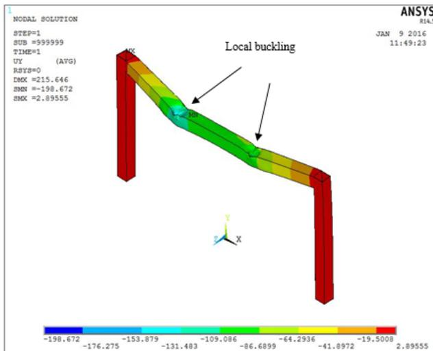
Fig. 8 Failure modes of FC0 FE model
