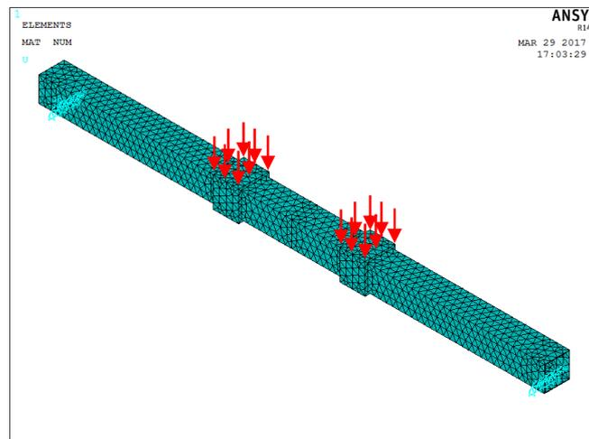
Fig. 3 Typical loading and boundary condition assigned to SHS steel beam in ANSYS
