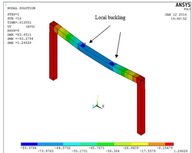
Fig. 9 Failure modes of FC2-1000-180 FE model
