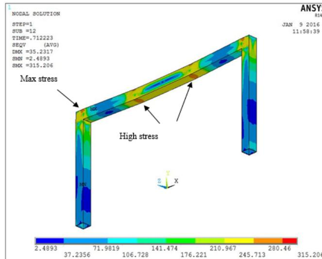
Fig. 6 Von Mises stress (FC0 FE model)
