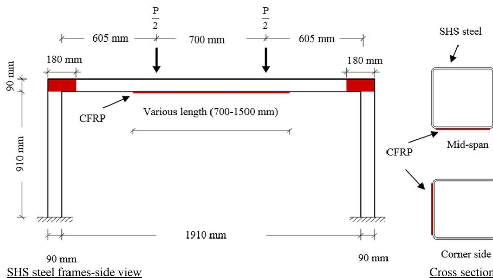
Fig. 5 Boundary conditions of a SHS steel frames strengthened with CFRP
