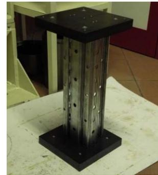
Fig. 5 Specimen ready for a stub-column test
