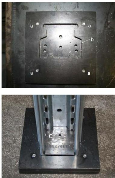
Fig. 4 Housing plates: (a) holes for bolts connecting the two plates of each couple; (b) hole with the profile perimeter in the upper plate; (c) inner plate to block section against inward distortion
