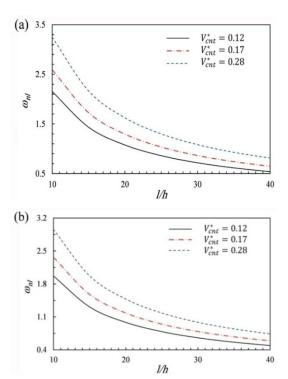
Fig. 5 Dimensionless nonlinear frequencies versus slenderness ratio for S-S CNTRC beams at a = 0.5: (a) UD; and (b) FG
