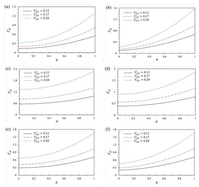
Fig. 7 Dimensionless post-buckling loads versus dimensionless maximum deflection of CNTRC beams with different volume fractions: (a) S-S UD; (b) S-S FG; (c) C-C UD; (d) C-C FG; (e) C-S UD; and (f) C-S FG
