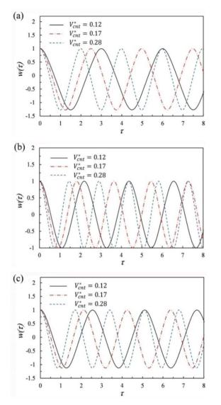
Fig. 4 Vibration response of FG-CNTRC beams at a = 1: (a) S-S; (b) C-C; and (c) C-S
