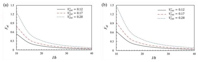
Fig. 8 Dimensionless post-buckling loads versus slenderness ratio for S-S CNTRC beams at a = 0.5: (a) UD; and (b) FG
