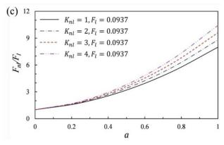
Fig. 9 Post-buckling load ratios versus dimensionless maximum deflection of S-S FG-CNTRC beams with  $V_{cnt}^* = 0.12$  for different values of foundation parameters: (a)  $K_l$  ( $K_s = K_{nl} = 0$ ); (b)  $K_s$  ( $K_l = K_{nl} = 0$ ); and (c)  $K_{nl}$  ( $K_l = K_s = 0$ )
