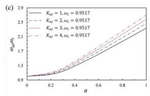
Fig. 6 Nonlinear frequency ratios versus vibration amplitude of S-S FG-CNTRC beams with  $V_{cnt}^* = 0.12$  for different values of foundation parameters: (a)  $K_l$  ( $K_s = K_{nl} = 0$ );(b)  $K_s$  ( $K_l = K_{nl} = 0$ ); and (c)  $K_{nl}$  ( $K_l = K_s = 0$ )
