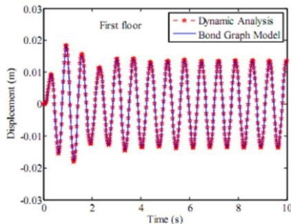
(a) Dynamic response of the frame to sinusoidal loading (Moustafa *et al.* 2007)
