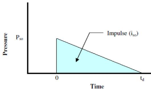
Fig. 5 Idealized shape of the blast load
