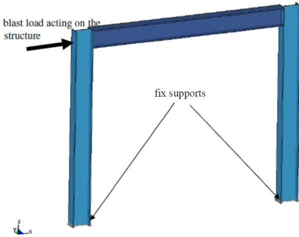
Fig. 4 The steel frame structural system
