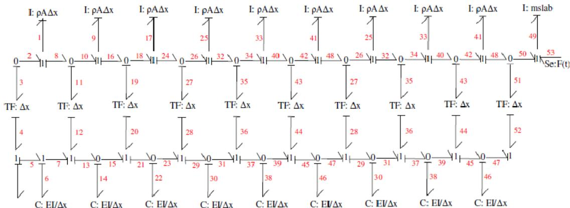
Fig. 7 The bond graph for the equivalent lump mass model
