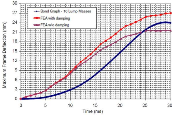
Fig. 10 Comparison of the maximum steel frame deflection time histories
