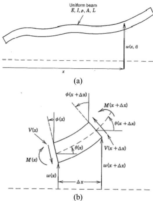
Fig. 2 Uniform beam in transverse motion (Karnopp *et al.* 1990)
