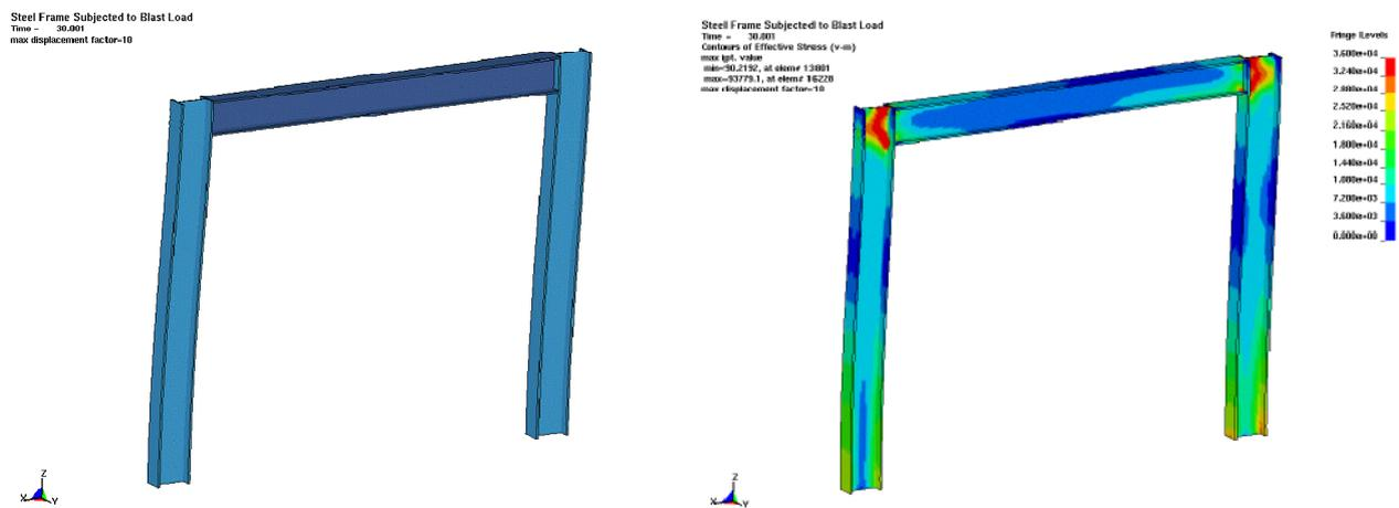
Fig. 9 Deflected finite element model and Effective stress distribution
