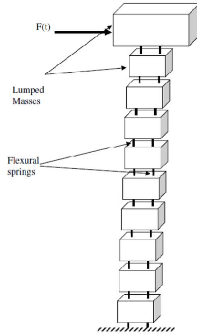
Fig. 6 The equivalent lump mass model used in bond graph modeling
