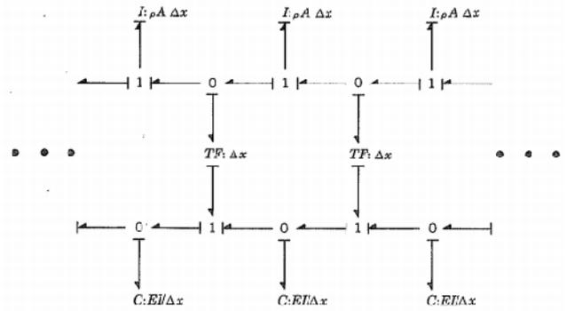
Fig. 3 Bond graph finite lump model of Bernoulli-Euler beam (Karnopp *et al.* 1990)
