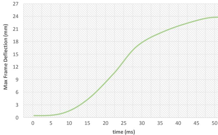
Fig. 8 Maximum steel frame deflection calculated using bond graph modeling with lump mass technique
