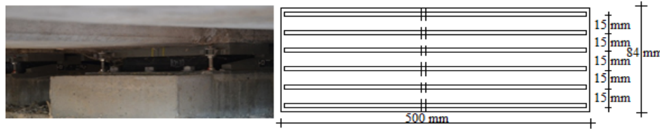
Fig. 4 Elastomeric bearing on abutments and its section properties
