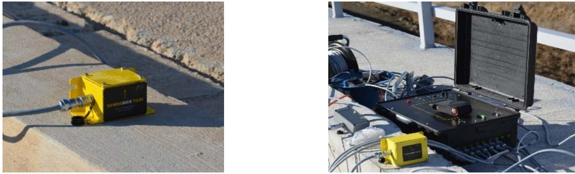
Fig. 6 Uni-axial accelerometer and data acquisition system used during ambient vibration testing of the bridges
