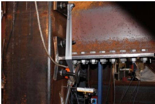
Fig. 17 Deformed shape of the T-flange at the ultimate load
