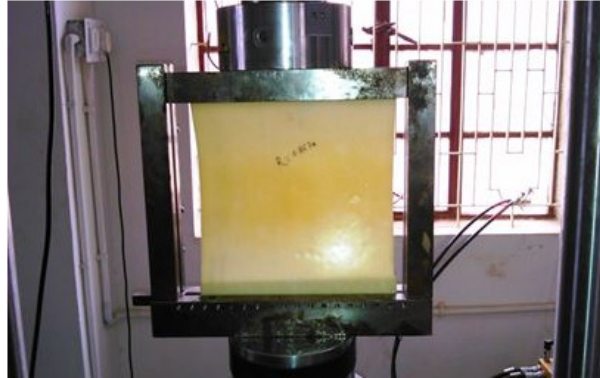
Fig. 6 Buckling test of CFCF laminated cylindrical shell panel on INSTRON 8862
