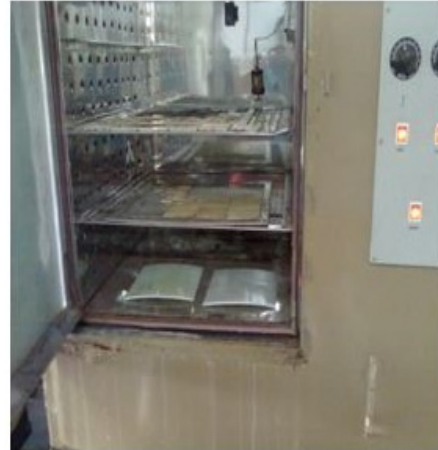
Fig. 5 Composite shell panels in humidity chamber
