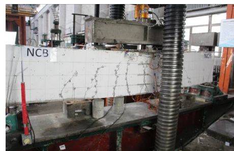
(b) NCB loading beyond cracking load
