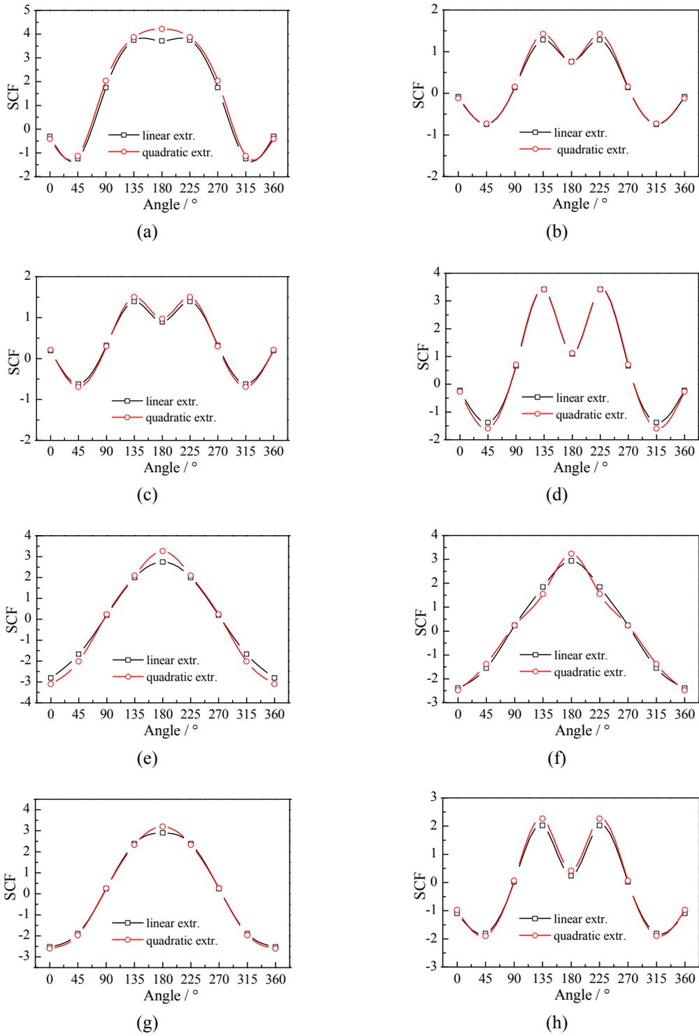
Fig. 4 Comparison of the SCFs obtained by linear and quadratic extrapolation: (a) SJ1 chord; (b) SJ2 chord; (c) SJ3 chord; (d) SJ4 chord; (e) SJ1 brace; (f) SJ2 brace; (g) SJ3 brace; (h) SJ4 brace
