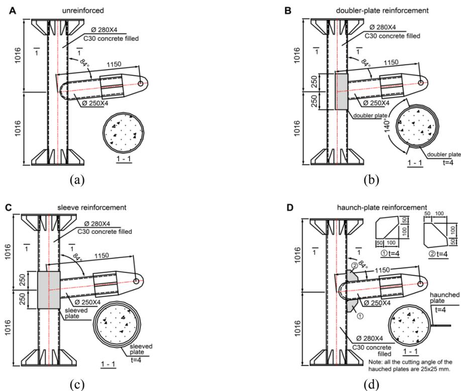
Fig. 1 Geometry of specimens (unit: mm): (a) unreinforced joint; (b) doubler-plated reinforcement; (c) sleeved reinforcement; (d) haunch-plated reinforcement
