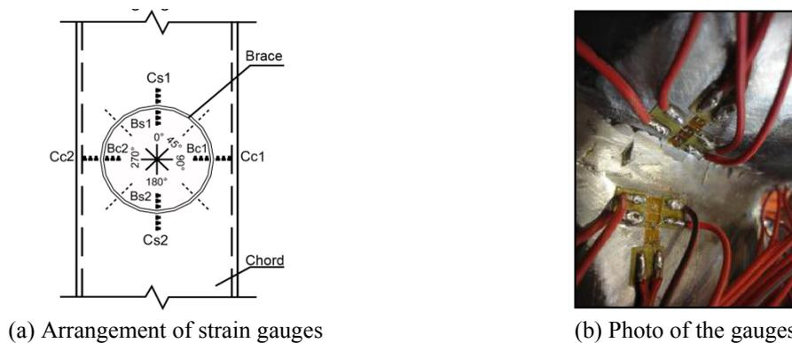
Fig. 3 Arrangement of strain gauges and test photo: (a) arrangement of strain gauges; (b) photo of gauges
