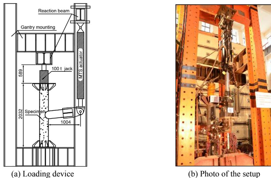
Fig. 2 Experimental setup: (a) loading device; (b) photo of setup
