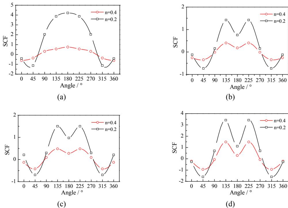
Fig. 6 Effect of the axial compression ratio on the SCF distributions in joints: (a) SJ1 chord; (b) SJ2 chord; (c) SJ3 chord; (d) SJ4 chord; (e) SJ1 brace; (f) SJ2 brace; (g) SJ3 brace; (h) SJ4 brace
