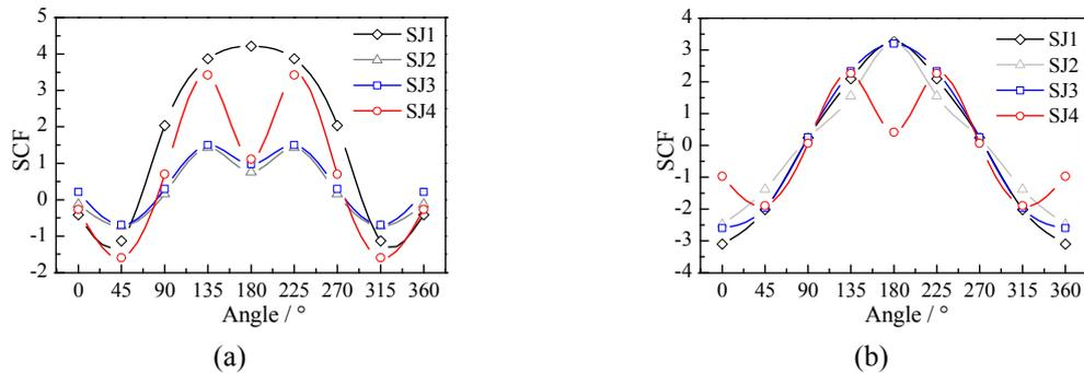
Fig. 5 Comparison of the SCF distributions in joints with different forms of reinforcement: (a) chord; (b) brace
