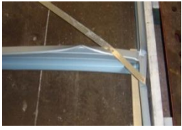
(c) Severe distortional buckling
