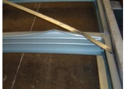
(b) Distortional buckling
