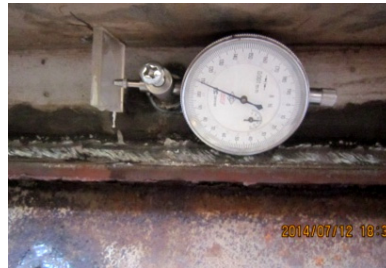
Fig. 9 Dial gauges for measuring PSS connector slip
