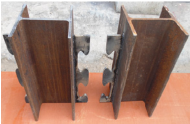
(b) Welded crestbond rib on steel beam
