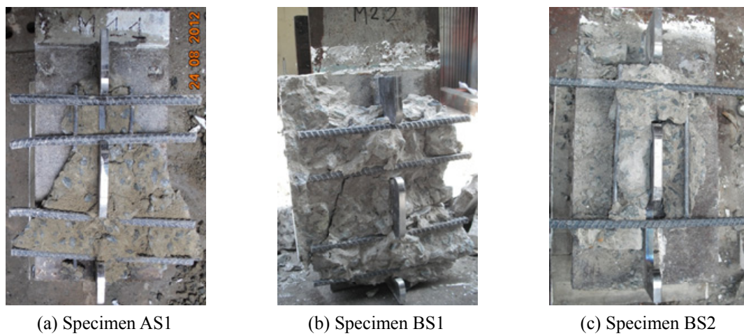
Fig. 11 Deformation of shear connectors and transverse rebars in crestbond holes
