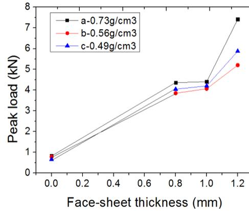
Fig. 8 Variation of peak load with face-sheet thickness
