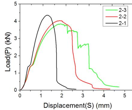
Fig. 3 Curve of S-P of AFS with the face-sheet of 0.8 mm
