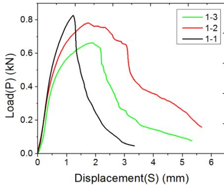
Fig. 2 Curve of S-P of foam only beams
