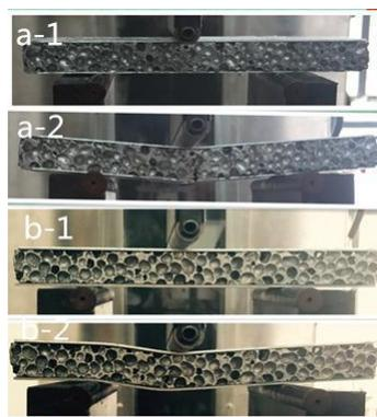
Fig. 9 AFS with 15 mm thick foam core and different face-sheet under three-point bending: (a) thin face-sheet with the value of 0.8 mm; (b) thick face-sheet with the value of 1.2 mm
