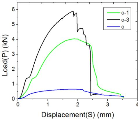
Fig. 7 Curve of S-P of AFS with the aluminum foam density of  $0.73 \text{ g/cm}^3$
