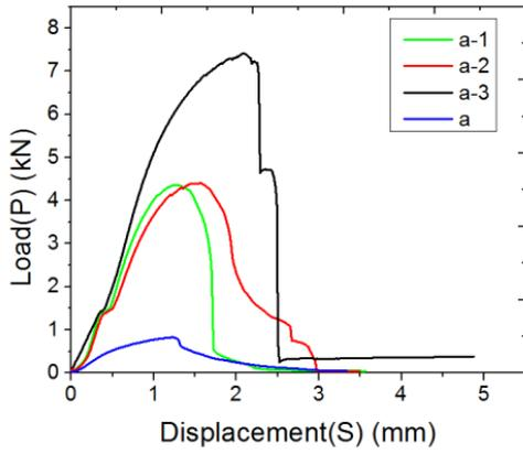
Fig. 5 Curve of S-P of AFS with the aluminum foam density of  $0.73 \text{ g/cm}^3$
