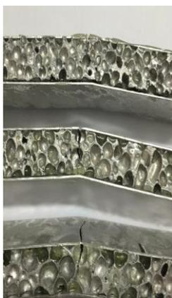
Fig. 10 Failure mode I
