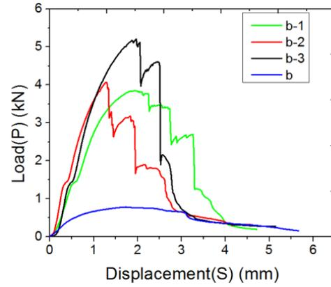
Fig. 6 Curve of S-P of AFS with the aluminum foam density of  $0.56 \text{ g/cm}^3$
