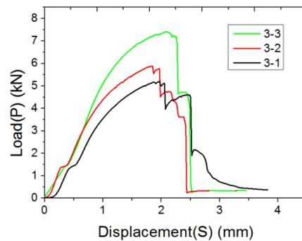
Fig. 4 Curve of S-P of AFS with the face-sheet of 1.2 in thickness mm
