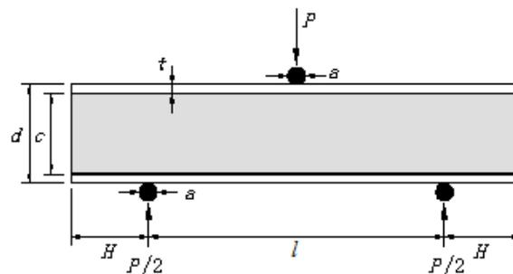
Fig. 1 Sandwich beam under three-point bending
