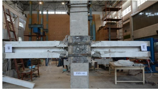
(b) PAN joint failure
