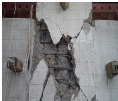
(g) RC-01 ultimate failure diagram
