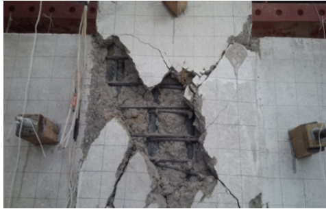
(a) RC-01 joint failure
