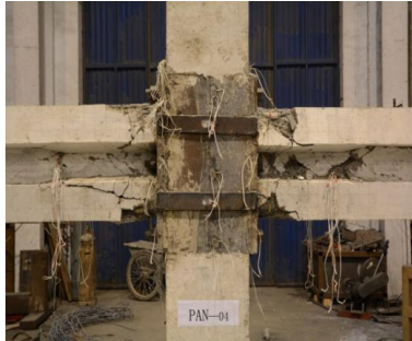
(a) PAN-04 ultimate failure diagram
