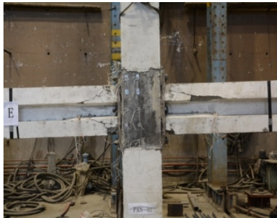
(c) PAN-03 ultimate failure diagram
