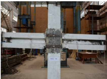
(e) PAN-06 ultimate failure diagram
