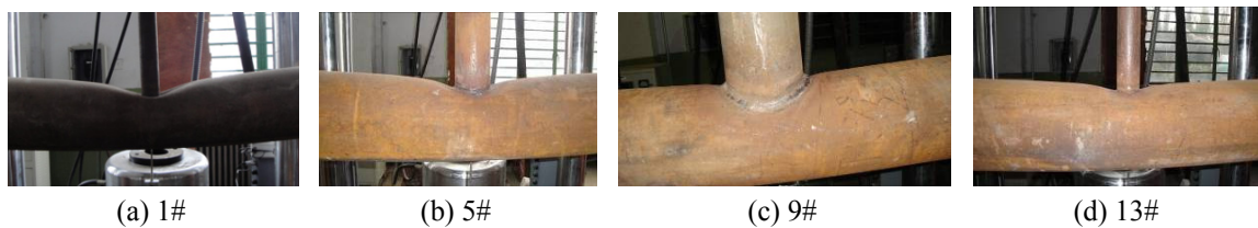
Fig. 3 Deformation of the un-reinforced specimens
