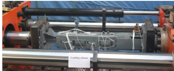
Fig. 14 Test system of PS-SCED brace
