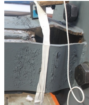
Fig. 18 Buckling of connecting plates of PS-SCED brace
